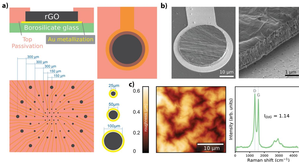
**Fig. 1** Fabrication and characterization of rGO MEAs. (a) Cross-section and top views of a microelectrode from the array, bottom panel shows the MEA design together with size and pitch of the electrodes. (b) SEM images showing the structure of a single microelectrode and the cross-section of the rGO structure before deposition of the top passivation layer. (c) Representative AFM image (left) and Raman spectrum (right) of the rGO microelectrode.
