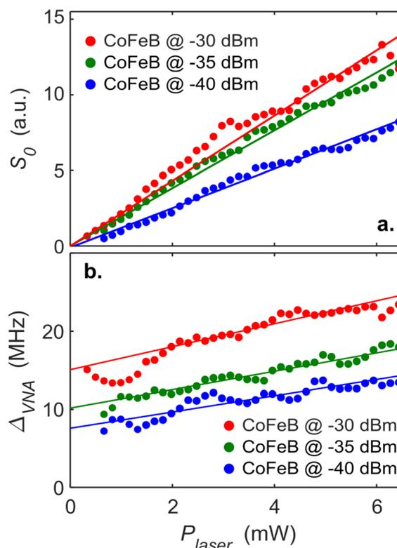
Fig. 5 Extracted (a)  $S_0$  and (b)  $\Delta_{\text{VNA}}$  vs.  $P_{\text{laser}}$  for the CoFeB SHNO. Solid lines represent linear fits to the data. The intercepts with  $P_{\text{laser}} = 0$  of the fits in b. are shown as pale blue stars in Fig. 4b and used to extract the intrinsic free-running SHNO linewidth ( $\Delta_f$ ).
