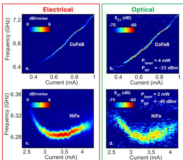
Fig. 2 Typical power spectral density (PSD) vs.  $I_{\text{DC}}$  measurements of CoFeB (a) and (b) and NiFe (c) and (d) SHNOs. The left column (a) and (c) shows traditional electrical measurements and the right column (b) and (d) shows the corresponding optical measurements. The applied field conditions were  $H = 3600$  Oe,  $\theta = 65^\circ$ , and  $\phi = 22.5^\circ$  for CoFeB and  $H = 6300$  Oe,  $\theta = 82^\circ$ , and  $\phi = 22.5^\circ$  for NiFe.
