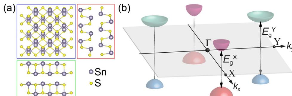
**Fig. 1** Crystal structure and band edges of orthorhombic SnS. (a) Crystal structure of SnS (space group  $Pnma$ ). Red, green, and blue boxes show views along  $[100]$ ,  $[010]$ , and  $[001]$  axes. (b) Schematic illustration of the valence- and conduction band edges of SnS along  $k_x$  and  $k_y$  reciprocal space axes, with bandgaps  $E_g^X$  and  $E_g^Y$  of the non-degenerate  $X$ - and  $Y$ -valleys, respectively.
