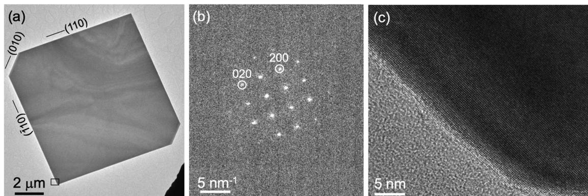
**Fig. 2** Structure and morphology of homogeneous SnS flakes. (a) TEM image of an entire SnS flake (side length 9.4  $\mu\text{m}$ ). (b) Nanobeam electron diffraction pattern of the flake, identifying the major side facets as {110} facets. (c) High-resolution TEM image showing SnS lattice fringes throughout the flake up to the free surface.
