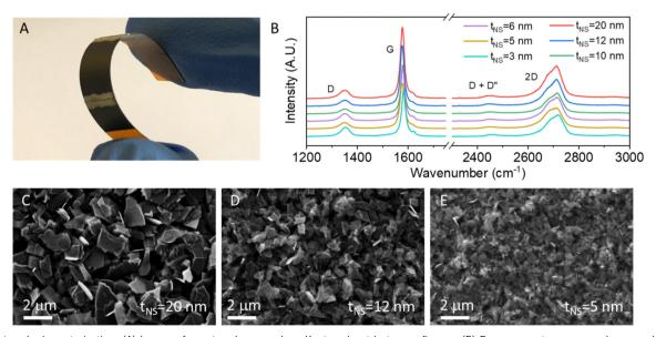
Fig. 2 Network characterisation. (A) Image of a network sprayed on Kapton, bent between fingers. (B) Raman spectra measured on graphene films sprayed from each size selected ink. (C)-(E) Top-down SEM of the networks of (C) large (0.5 to 1 kRPM) and (D) medium (1.5 to 2 kRPM) and (E) small (3 to 4 kRPM) size selected nanosheets. In (C)–(E) the mean nanosheet thickness,  $t_{NS}$ , is given in the panel.
