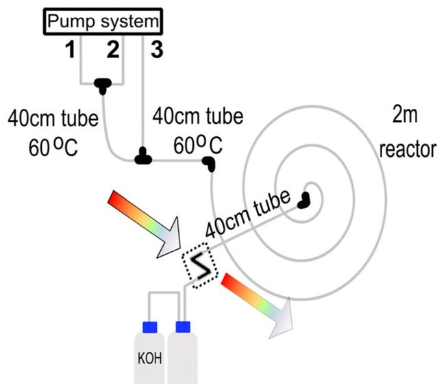
**Fig. 3** Schematic representation of the microfluidic reactor designed to produce Prussian blue nanoparticles. Pump channels chemicals  $\rightarrow$  1 = citric acid [25.5 mM]; 2 =  $\text{FeCl}_3$  [1 mM]; 3 =  $\text{K}_4[\text{Fe}(\text{CN})_6] \cdot 3\text{H}_2\text{O}$  [1 mM] + citric acid [25.5 mM].
