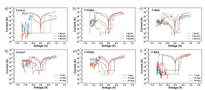
Fig. 4 Resistive switching device stability. I-V characteristics of the devices (a)-(c) for 3 months under inert atmosphere and (d)-(f) for 40 days in ambient air, including control (a) and (d), F-PDMAI<sub>2</sub> (b) and (e) and F-BNAI (c) and (f) treated devices. Complementary device stability is shown in Fig. S11 and S12 of the ESI.†
