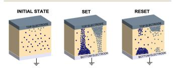
Fig. 5 Resistive switching mechanism. Schematic of the resistive switching of halide perovskite memory devices, indicating the formation (SET) and rupture (RESET) of the conductive filaments (ion vacancies in blue and metal cations in grey). The perovskite layer is represented in light orange.
