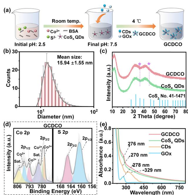
Fig. 2 Glucose oxidase-carbon dots- $\text{CoS}_x$  QD (GCD/CO) nanodevice characterization. (a) Synthesis schematic of GCD/CO. (b) Particle size distribution of GCD/CO. (c) XRD spectra, and (d) XPS spectra showing an unaffected structure of  $\text{CoS}_x$  QDs in GCD/CO. (e) UV-vis absorption spectra of GCD/CO,  $\text{CoS}_x$  QDs, CDs and GOx.
