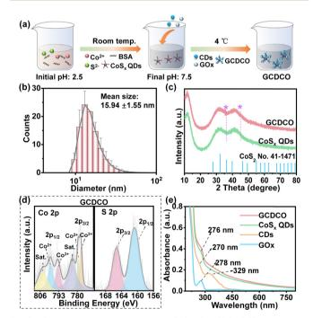
Fig. 2 Glucose oxidase-carbon dots- $CoS_x$  QD (GCDCO) nanodevice characterization. (a) Synthesis schematic of GCDCO. (b) Particle size distribution of GCDCO. (c) XRD spectra, and (d) XPS spectra showing an unaffected structure of CoS<sub>x</sub> QDs in GCDCO. (e) UV-vis absorption spectra of GCDCO, CoS<sub>x</sub> QDs, CDs and GOx
