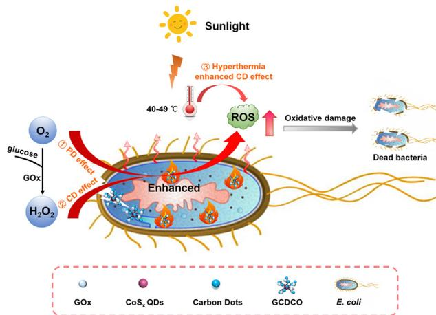
Fig. 1 Schematic illustration of cascade bioreactor GDCO for achieving the hyperthermia-enhanced CD/PD effect and GOx-catalysis-enhanced CD effect of bacterial inactivation.
