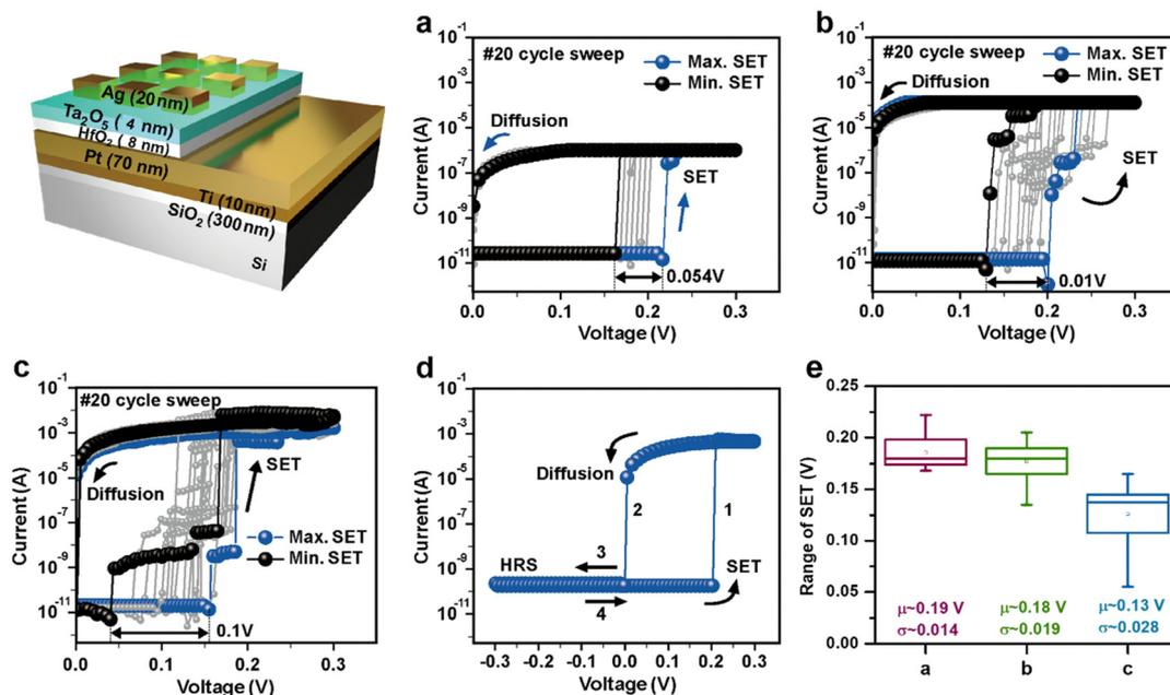
Fig. 2 The schematic diagrams and the  $I$ - $V$  curve of the  $\text{Ta}_2\text{O}_5/\text{HfO}_2$  hybrid device with different compliance currents; (a)  $10^{-6}$  A, (b)  $10^{-4}$  A, and (c) no compliance current. (d) The maintenance of a high resistance level during the application of the negative DC sweep. (e) The calculated average,  $\mu$  and standard deviation,  $\sigma$  for different compliance current levels from (a) to (c).
