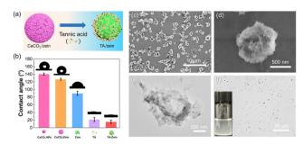
Fig. 3 (a) Schematic representation of the procedure for tannic acid (TA) treatment. (b) The water contact angle of the hydrophobic  $CaCO_3$  nanoparticles, the  $CaCO_3$ /zein microparticles, zein powder, tannic acid powder, and TA/zein microparticles. SEM images (c), (d) and TEM image (e) of the TA/zein microparticles. (f) Picture and optical microscopy image of the water-dispersed TA/zein microparticles.
