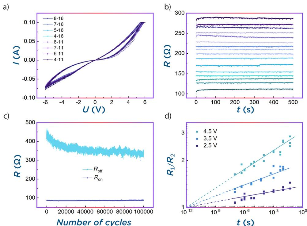
**Fig. 2** Memristive characteristics of the CFB-LNO NC-based crossbar array. (a) Current–voltage characteristics of eight memristors from the  $16 \times 16$  crossbar array; (b) retention of 16 stable resistive states, and (c) endurance over  $10^5$  consecutive resistive switching events of a single CFB-LNO NC memristor; (d) dependence of the initial ( $R_1$ ) to final ( $R_2$ ) resistance ratio vs. duration of switching pulse at different voltage amplitudes.
