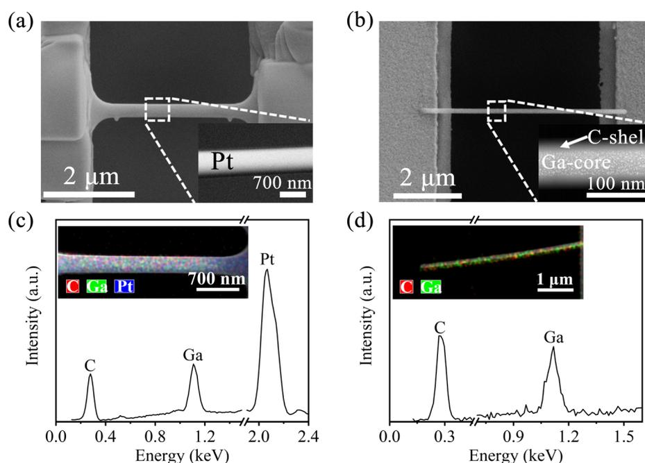
Fig. 5 SEM image of the (a) Pt nanopillar and (b) C nanowire fabricated by FIB. The insets are STEM images of the Pt nanopillar and C nanowire. EDS analysis of the (c) Pt nanopillar and (d) C nanowire.
