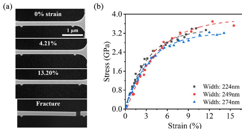
Fig. 6 Sequential SEM images (a) and strain–stress curves (b) of the Pt nanopillar during tension to fracture.
