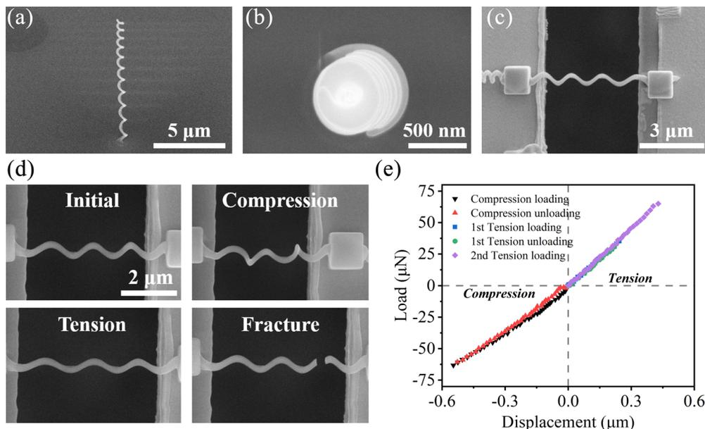
**Fig. 10** The front (a) and top view (b) SEM images of the C nanospring fabricated by FIB 3D nanoprinting. (c) SEM image of the nanospring transferred and fixed by a nanomanipulator and EBID. (d) A series of SEM images of the C nanowire during the tension–compression test. (e) The load–displacement curve of the C nanospring.
