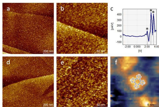
Fig. 3 STM images ( $U_B = 2$  V;  $I_T = 10$  pA) of a (PcDy)<sub>2</sub>-POV12 layer (a) and (b) with corresponding *dI/dV* curve (c) measured on a single point in (b) and of a PcDyOAc layer (d) and (e). High resolution imaging of a single PcDyOAc molecule (f) exhibits Pc characteristic fourfold symmetry indicated by the overlay of a calculated metal Pc LUMO structure.<sup>43</sup>
