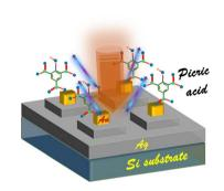
3D nanoplasmonic structure for ultrahigh enhanced SERS with less variability, polarization independence, and multimodal sensing applied to picric acid detection
