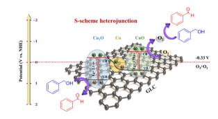
Synergistic atom co-sharing and S-scheme heterojunction: constructing Cu/CuO/Cu<sub>2</sub>O with ultrathin graphene-like carbon derived from basil seeds for enhanced photo-oxidation of benzyl alcohols to aldehydes
