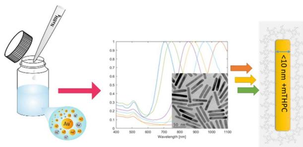
**High yield seedless synthesis of mini gold nanorods: partial silver decoupling allows effective nanorod elongation with tunable surface plasmon resonance beyond 1000 nm and CTAB-free functional coating for *m*THPC conjugation**
