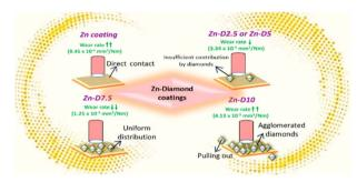
Nanodiamond-structured zinc composite coatings with strong bonding and high load-bearing capacity
