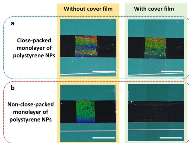
Fig. 2 Labels with (a) close-packed, and (b) non-close-packed monolayer of polystyrene NPs on black tape before and after application of a transparent cover film (scale bar: 1 cm).
