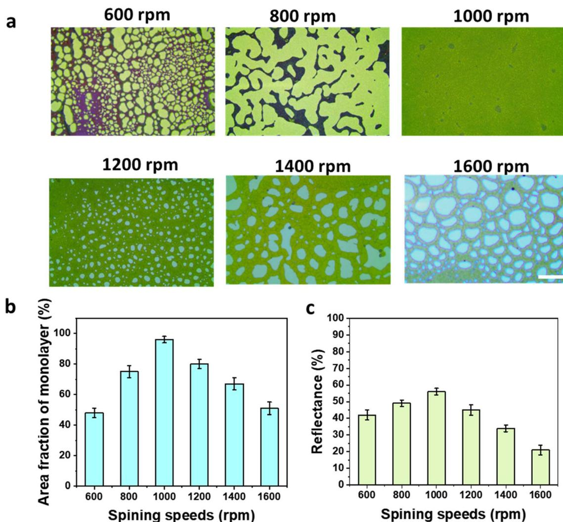
Fig. 8 (a) Optical microscopy images of particle layers on a silicon substrate for various spin speeds (scale bar: 100  $\mu\text{m}$ ), (b) area fraction of monolayers and (c) reflectance of particle layers for various spin speeds.
