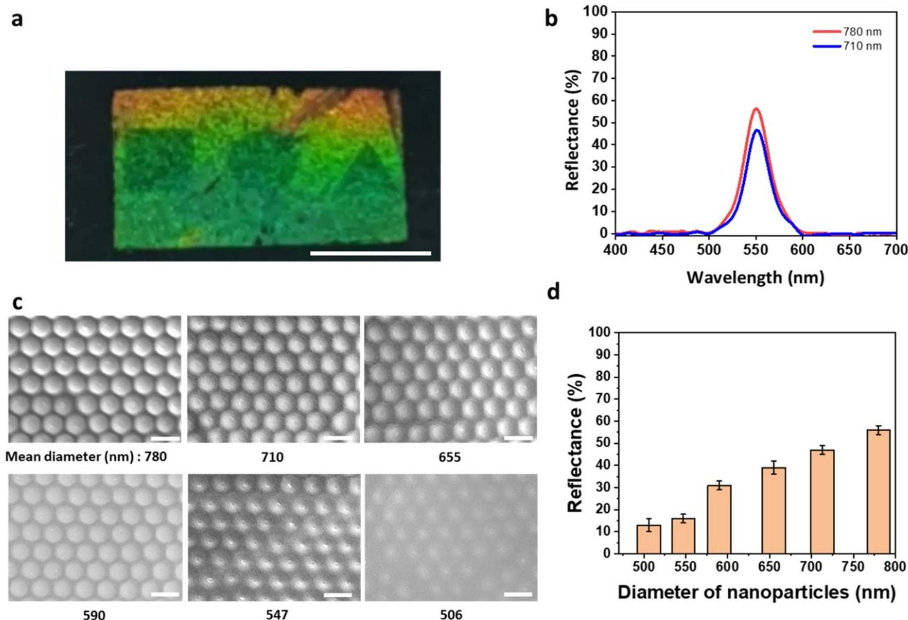
Fig. 7 (a) Photo (scale bar: 1 cm) and (b) reflectance spectrum of PCs with identical lattice constants but different particle diameters. (c) SEM images of various monolayers of PCs (scale bar: 1 μm) and (d) their reflectance. All PCs were fabricated on a black adhesive tape.
