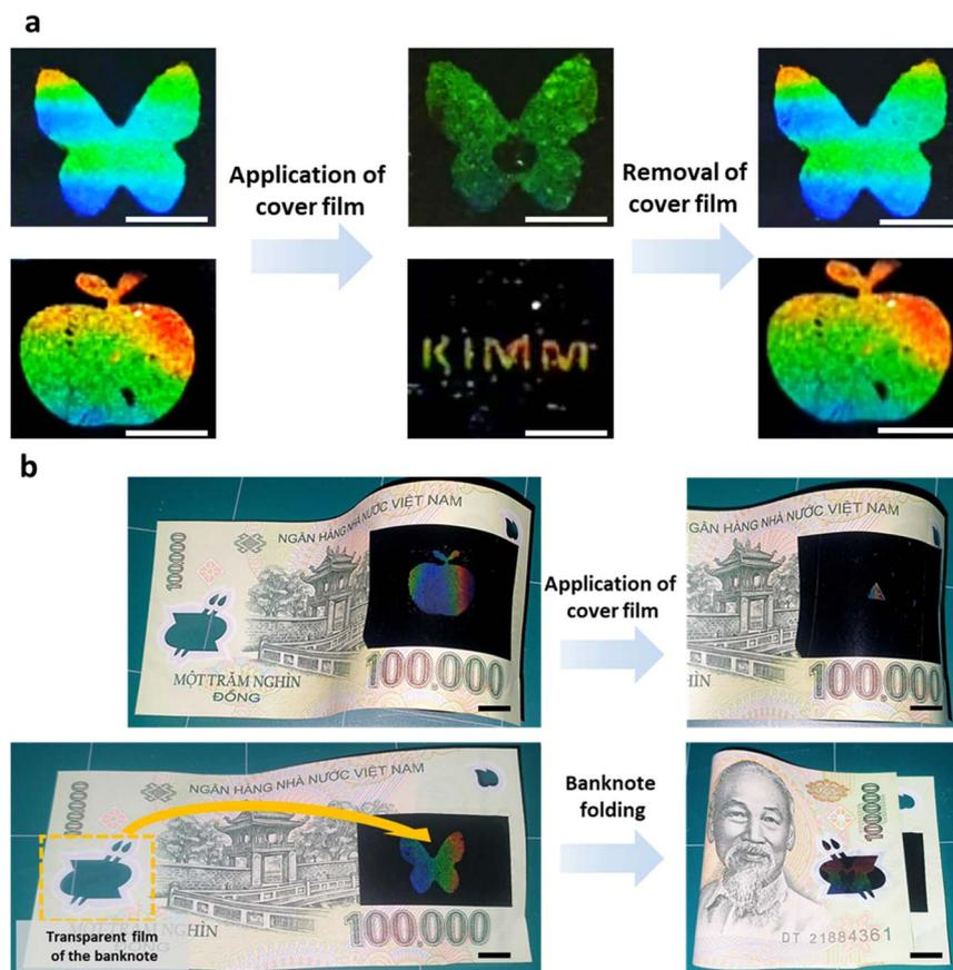
Fig. 9 (a) Hybrid labels containing the CPM and NCPM, (b) the hybrid labels on a Vietnamese banknote at a bent state (top image) and flat state (bottom image) (scale bar: 1 cm).
