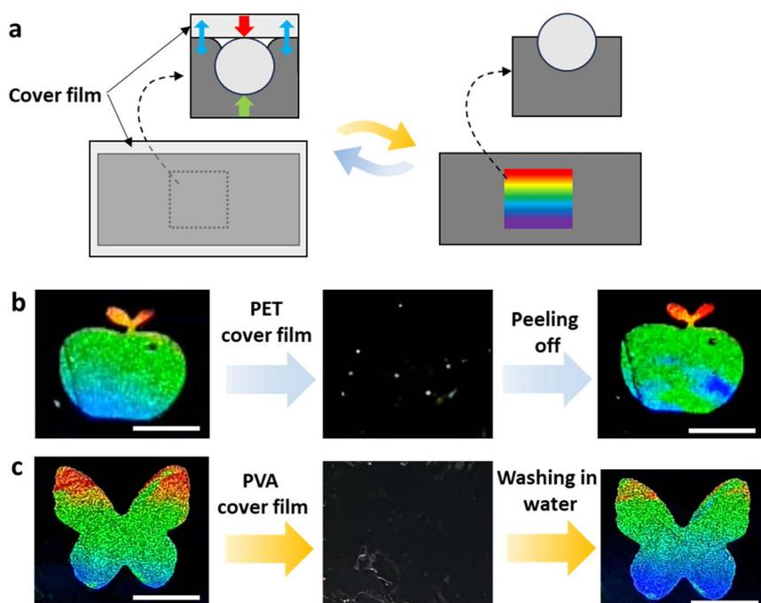
Fig. 4 (a) Illustration of embedding or extrusion of nanoparticles on adhesive tape, (b) revelation of the label by peeling off the cover film, and (c) revelation of the label by dissolving the cover film (scale bar: 1 cm).
