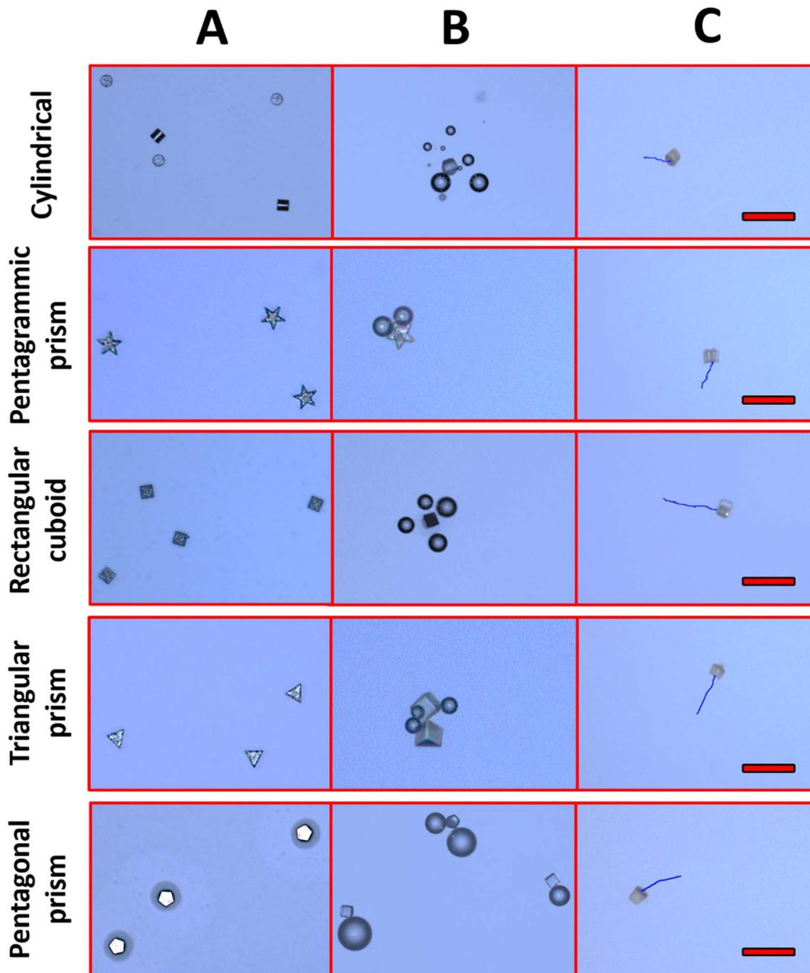
Fig. 3 Optical imaging of Zn/SU-8 MMs (A) before acid addition, (B) bubble formation after acid addition (1 M HCl, 1.3% Triton X-100), (C) tracking over time duration of 5 s. Scale bars: 100  $\mu\text{m}$ .
