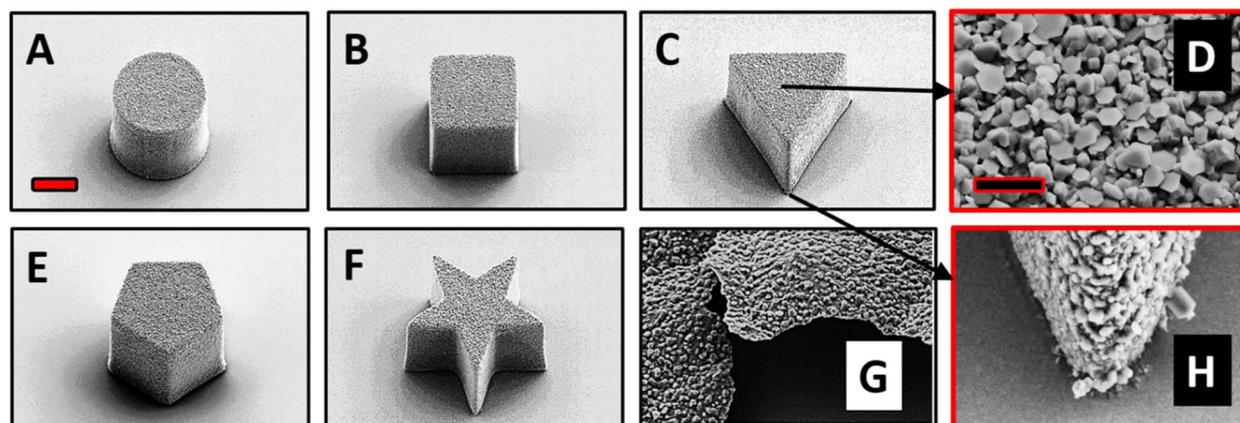
Fig. 1 Characterization of Zn/SU-8 MMs. SEM image of (A) cylindrical, (B) rectangular cuboid, (C) triangular prism, (D) top view of triangular prism, (E) pentagonal prism, (F) pentagrammic prism, (G) Zn film and (H) bottom view of triangular prism MMs.
