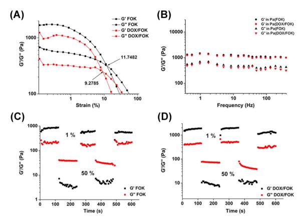
Fig. 4 (A) Dynamic strain sweep of FOK and DOX/FOK hydrogels. (B) Dynamic frequency scanning of FOK and DOX/FOK hydrogels. Circle sweep of (C) FOK and (D) DOX/FOK hydrogels.
