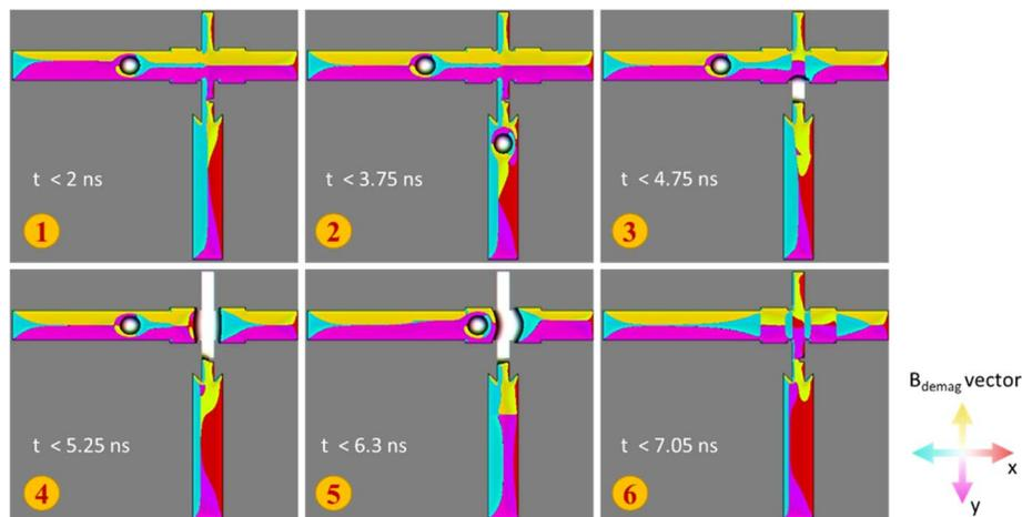
Fig. 2 Demagnetization field ( $B_{\text{demag}}$ ) spatial distribution at the different stages of the inverter gate operation is shown for the bottom interface. One layer in the SAF provides the mirrored response of the other.
