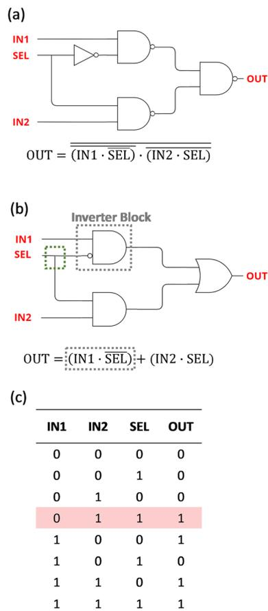
Fig. 7 2-To-1 multiplexer (MUX) circuit demonstration using the SAF logic inverter and duplicator blocks. (a) The initial circuit schematic of the MUX using the NAND and NOT gates with its Boolean function is simplified in (b) to demonstrate its function with the minimum number of inverter blocks and a duplicator block. The green shaded box represents the duplicator gate block shown in Fig. 8. (c) The truth table of the MUX Boolean function in (a) and (b).
