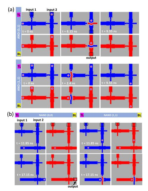
Fig. 5 Logic (a) AND and (b) NAND gates constructed by cascading and rotating the inverter blocks. Both gates' logic inputs (0, 0) and (1, 1) are demonstrated here.
