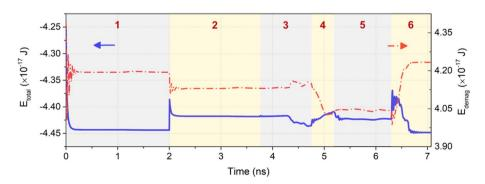
Fig. 3 SAF skyrmion inverter gate energy response plot shows the total energy ( $E_{total}$ ) and demagnetizing energy ( $E_{demag}$ ) time response during the gate operation.
