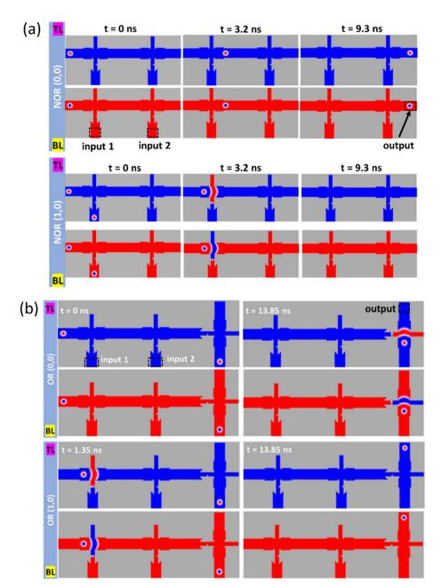
Fig. 4 Logic (a) NOR gate, of inputs (0, 0) and (1, 0), and (b) OR gate, of inputs (0, 0) and (1, 0), constructed from the inverter blocks showing the different stages of the SAF skyrmion input signals and probing skyrmions of the top and bottom layers transitions which lead to the output logic of the respective gates (BL: bottom layer, TL: top layer).
