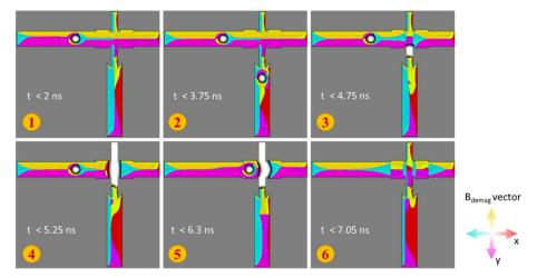
Fig. 2 Demagnetization field ( $B_{demag}$ ) spatial distribution at the different stages of the inverter gate operation is shown for the bottom interface. One layer in the SAF provides the mirrored response of the other.
