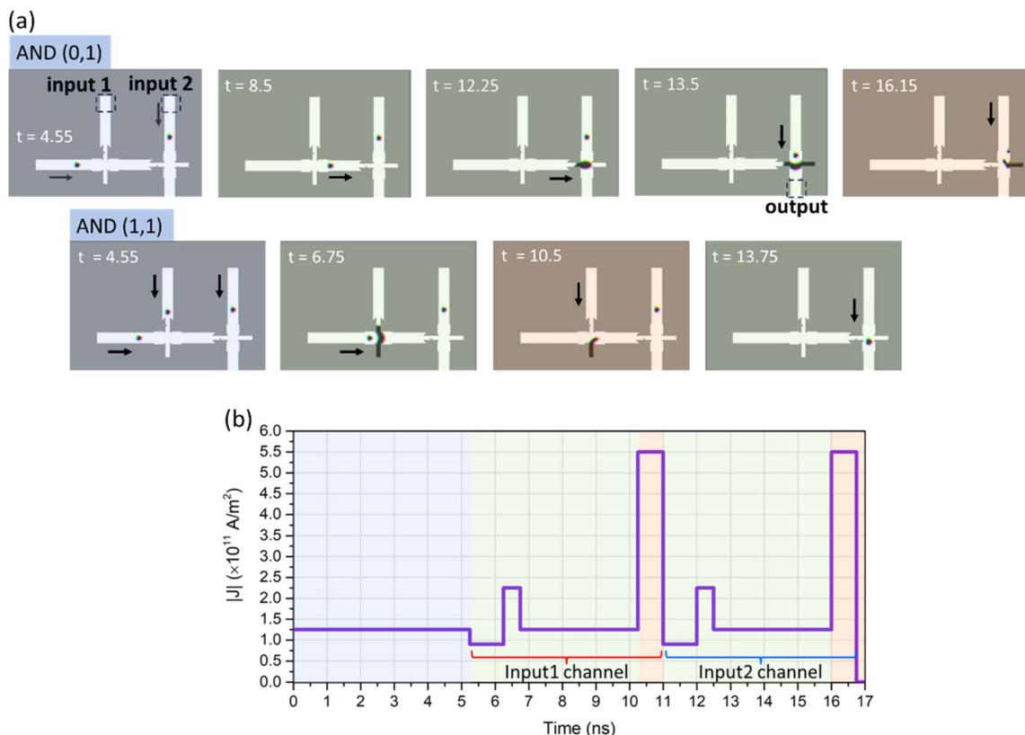
Fig. 6 The operation of the two-input SAF logic AND gates with inputs (0, 1) and (1, 1), respectively. (a) Snapshots of the different stages that are driven by applied current densities according to the timed plots in (b). The arrows show the direction of the applied current.
