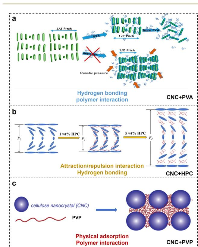
Fig. 6 Illustration showing the interactions between CNCs with different polymers: (a) PVA,<sup>101</sup> Copyright 2019, American Chemical Society; (b) HPC,<sup>104</sup> Copyright 2020, Elsevier; and (c) PVP,<sup>107</sup> Copyright 2023, American Chemical Society.
