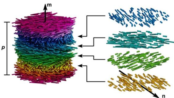
Fig. 3 Illustration of a cholesteric liquid crystal phase of densely packed CNCs. CNCs have local nematic-like ordering with a director  $n$  that rotates in a left-handed helicoid manner about the helical axis  $m$ . The cholesteric pitch,  $p$ , corresponds to a full  $360^\circ$  rotation of the director.<sup>31</sup> Copyright 2023, American Chemical Society.
