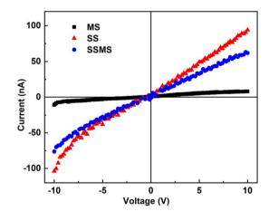
Fig. 9 /-V characteristics of SS, MS, and SSMS samples.
