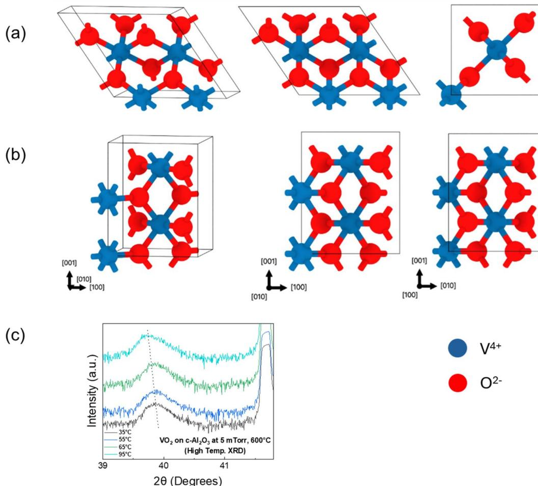
**Fig. 6** Schematic of the  $\text{VO}_2$  in bulk mode for (a) monoclinic and (b) tetragonal phases, and (c) the corresponding experimental results of high temperature X-ray diffraction, with the shift in the  $2\theta$  value confirming the transition at high temperatures.
