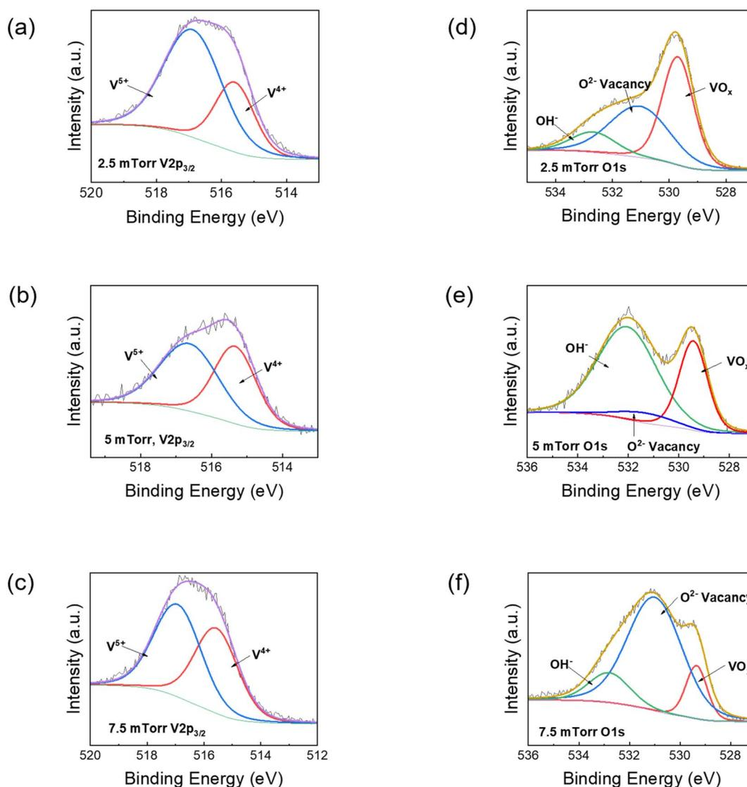
Fig. 3 XPS plots of the VO<sub>2</sub> samples deposited on (0001) Al<sub>2</sub>O<sub>3</sub> – (a, b and c) the de-convolution of V 2p peaks for VO<sub>2</sub> films formed at varying oxygen pressure levels (substrate temperature being 600 °C), and (d, e and f) the de-convoluted XPS data points of the O 1s level corresponding to the V 2p peaks in (a), (b) and (c) respectively.
