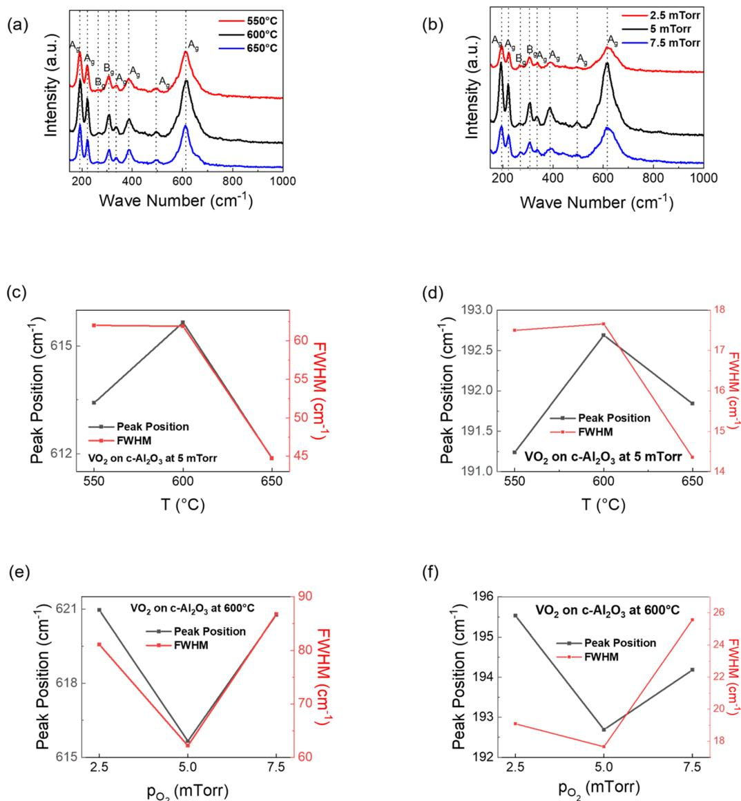
Fig. 4 Raman analysis of the VO<sub>2</sub> samples – (a) the Raman analysis of the substrate temperature-wise, and (b) the variation in Raman plot with change in oxygen pressure during deposition; (c and d) the respective FWHM and position of the main V–O and V–V stretching peaks with respect to deposition temperature respectively, and (e and f) oxygen pressure-wise comparison for the V–O and V–V peaks respectively.
