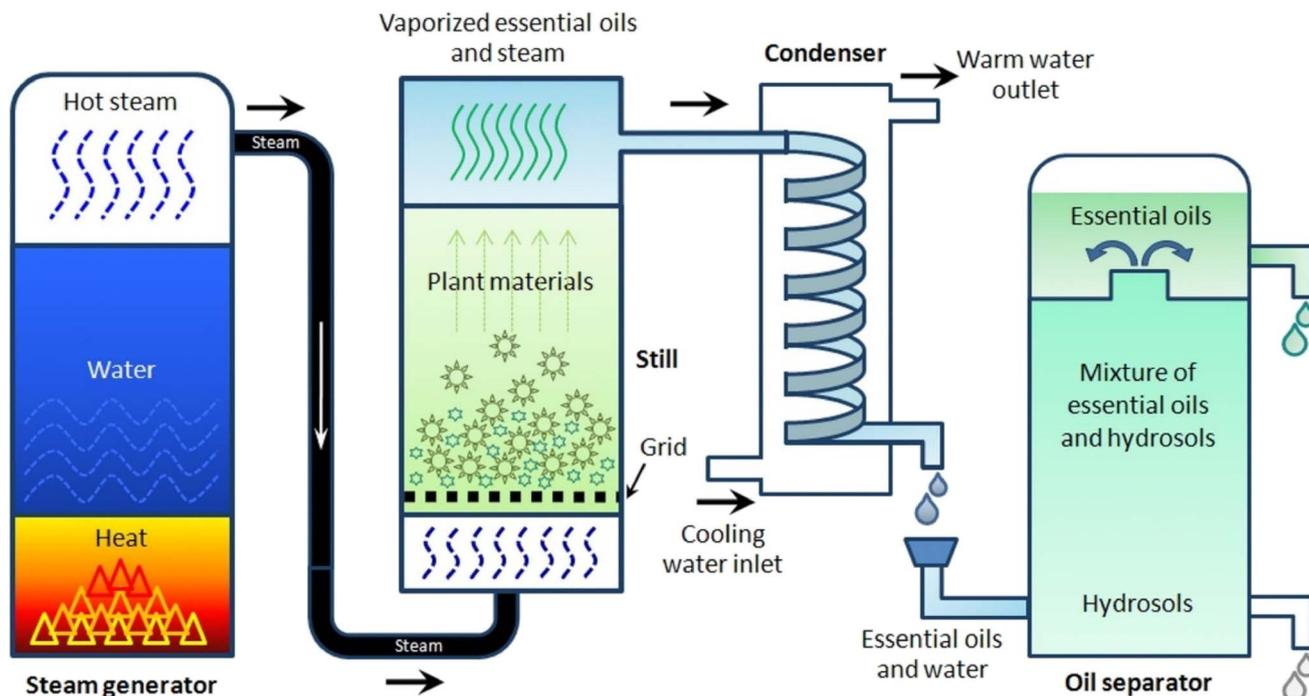
Fig. 3 Schematic representation depicts the steam distillation extraction method (process steps and main parts) utilized for EO extraction.<sup>47</sup> Reproduced with permission from ref. 47 Copyright 2014 John Wiley & Sons.
