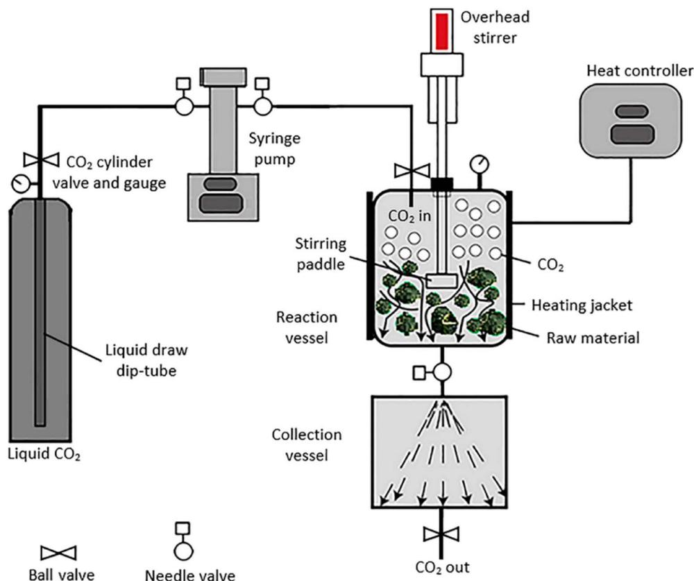
Fig. 4 The standard system of a supercritical fluid device.<sup>48</sup> Reproduced from ref. 48 Copyright 2017 MDPI.
