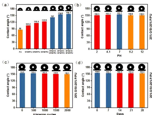
Fig. 4 The contact angle test graphs of the different experimental groups (a). The contact angle graphs after two weeks of immersion in various acid and alkali solutions (b). The contact angle graphs after different friction cycles (c). The contact angle graphs after different days of outdoor exposure (d).
