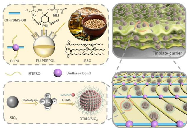
Fig. 1 The preparation process of the composite coating films.
