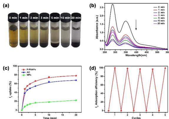
**Fig. 2** (a) Photograph showing solution color change when 6.0 mg of P-P6APs was placed in  $I_2/KI$  (aq) (250 ppm). (b) Time-dependent UV/vis absorption spectra of  $I_2/KI$  (aq) (250 ppm) upon addition of P-P6APs (6.0 mg). (c) Time-dependent  $I_2$  uptake efficiency based on the absorption peak at 286 nm after adding P-P6APs, AC and MPs. (d) Iodine adsorption efficiency of P-P6APs after the same material is recycled 5 times in  $I_2/KI$  (aq).
