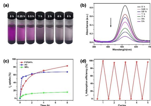
**Fig. 3** (a) Photograph showing color change when 24.0 mg of P-P6APs was placed in an iodine/ $n$ -hexane solution (1 mM). (b) Time-dependent UV/vis absorption spectra of an iodine/ $n$ -hexane solution (1 mM) upon addition of P-P6APs (24.0 mg). (c) Time-dependent  $I_2$  uptake efficiency based on the absorption peak at 522 nm after adding P-P6APs, AC and MPs. (d) Iodine adsorption efficiency of P-P6APs after the same material was recycled 5 times in an iodine/ $n$ -hexane solution.
