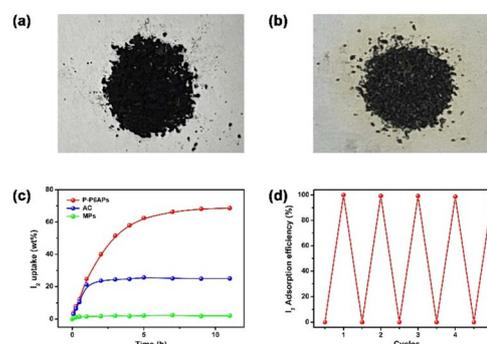
**Fig. 4** Photos of P-P6APs (a) before and (b) after exposure to iodine vapor for 11 h. (c) Time-dependent  $I_2$  vapor uptake efficiency of P-P6APs, AC and MPs at 80 °C. (d) Iodine adsorption efficiency of P-P6APs after the same material is recycled 5 times for iodine vapor capture.
