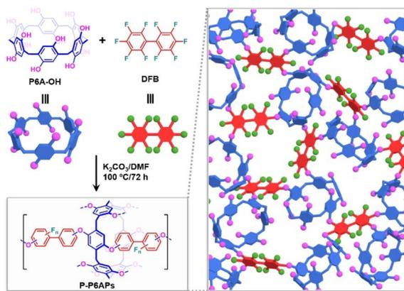
**Scheme 1** Pillar[6]arene-based polymer networks derived from nucleophilic aromatic substitution reactions. Left: Synthesis of the high-surface-area porous P-P6APs from P6A-OH and DFB. Right: Schematic of the P-P6APs structure.
