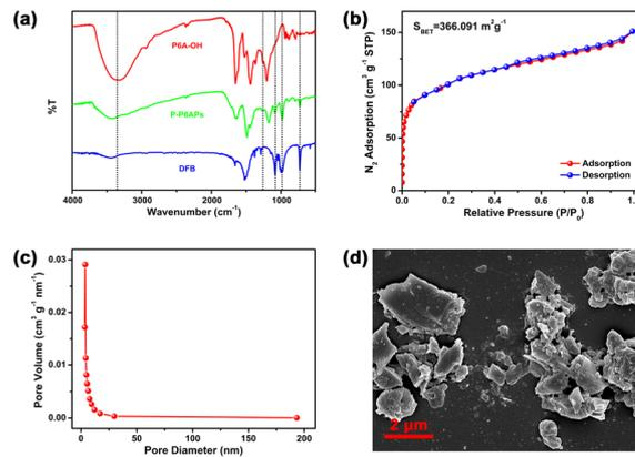
**Fig. 1** (a) FT-IR spectra of P6A-OH, P-P6APs and DFB. (b) Nitrogen adsorption/desorption isotherm of P-P6APs. (c) The cumulative pore volume (pore diameter) of P-P6APs obtained *via* a Barrett–Joyner–Halenda analysis. (d) SEM image of P-P6APs.
