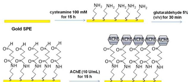
Fig. 21 Assembly process of the AChE biosensor. Reproduced from ref. 68 with permission from [Elsevier], copyright [2013].
