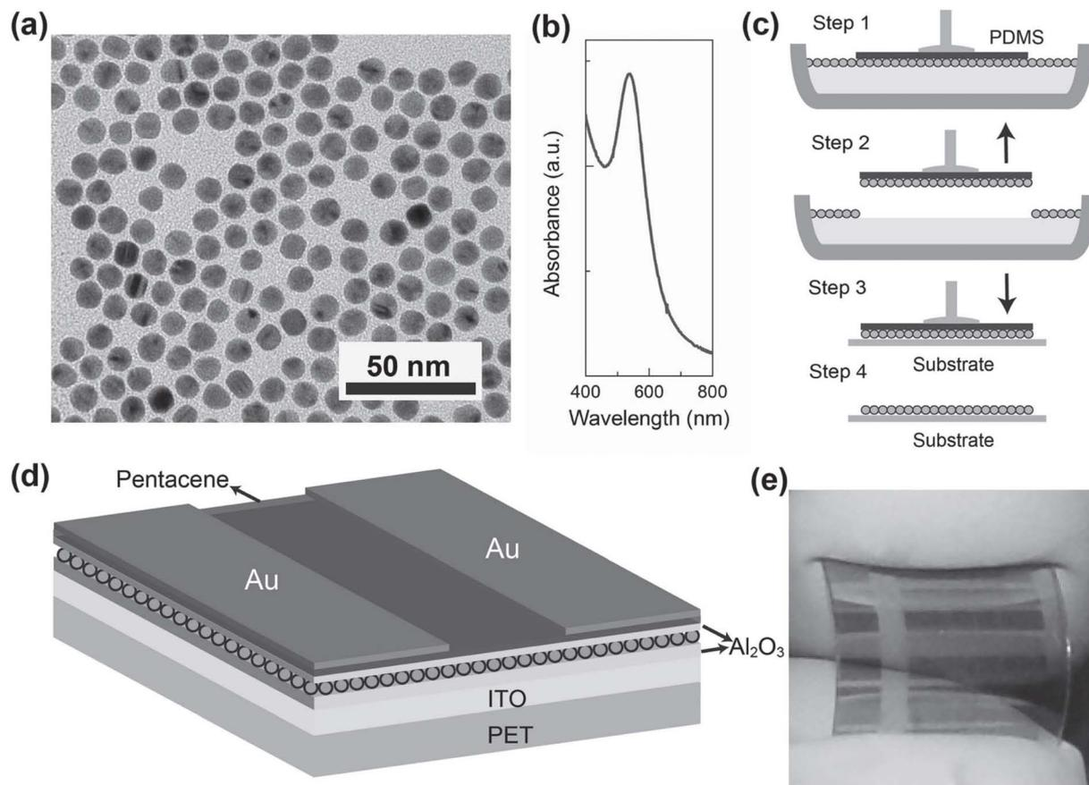
Fig. 13 Presents: (a) TEM image of 10 nm Au NPs coated with DDT. (b) UV-visible absorption spectra of Au-NPs in toluene. (c) Schematic process of forming NPs array on a substrate. (d) 3D schematic of the memory device architecture. (e) Optical photo of the fabricated flexible memory device. Reproduced from ref. 50 with permission from [Wiley], copyright [2012].
