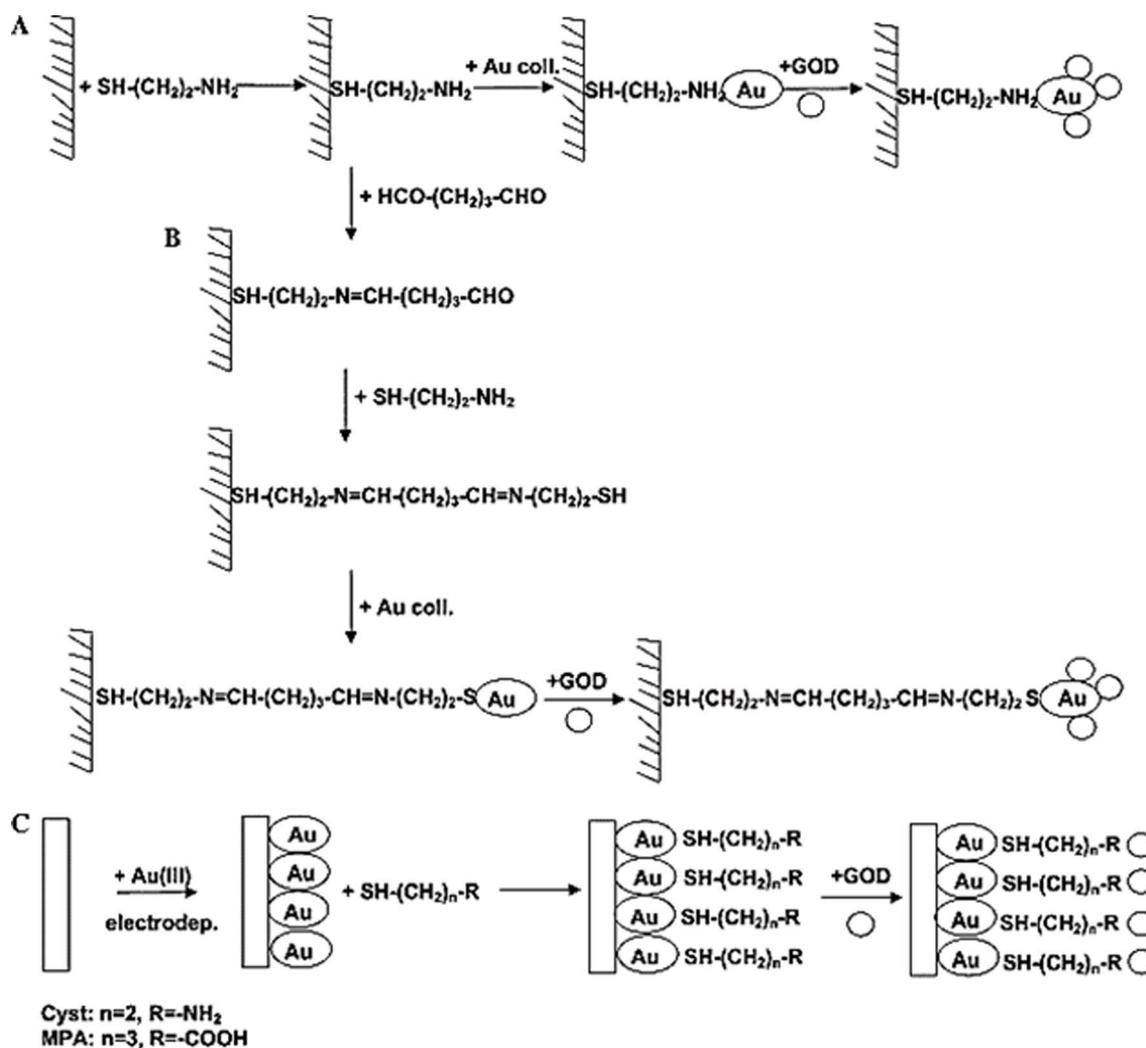
Fig. 20 Preparation strategies for glucose oxidase biosensors using gold nanoparticle-modified electrodes: (A)  $\text{GO}_x/\text{Au}_{\text{coll}}\text{-Cyst-AuE}$ , (B)  $\text{GO}_x/\text{Au}_{\text{coll}}\text{-Cyst/Cyst-AuE}$ , (C)  $\text{GO}_x/\text{Cyst-nAu-GCE}$  or  $\text{GO}_x/\text{MPA-nAu-GCE}$ . Reproduced from ref. 67 with permission from [Elsevier], copyright [2005].
