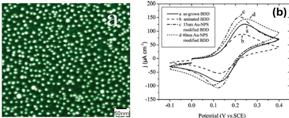
Fig. 17 (a) SEM images of amine-terminated BDD surfaces exposed to 15 nm Au-NP solutions for 6 hours. (b) CVs of 1 mM  $\text{Fe}(\text{CN})_6^{3-/4-}$  in 0.1 M  $\text{Na}_2\text{SO}_4$  at  $50 \text{ mV s}^{-1}$  for (a) as-grown BDD, (b) amine-terminated BDD, (c) 15 nm Au-NPs on BDD, and (d) 40 nm Au-NPs on BDD. Reproduced from ref. 61 with permission from [ACS Publications], copyright [2006].
