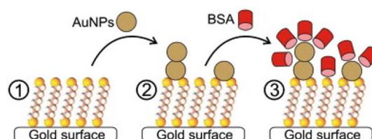
Fig. 24 Fabrication process of the SPR biosensor: formation of 1,10-DDT SAM on gold, chemisorption of Au-NP to 1,10-DDT SAM, immobilization of BSA on AuNP. Reproduced from ref. 73 with permission from [Elsevier], copyright [2009].
