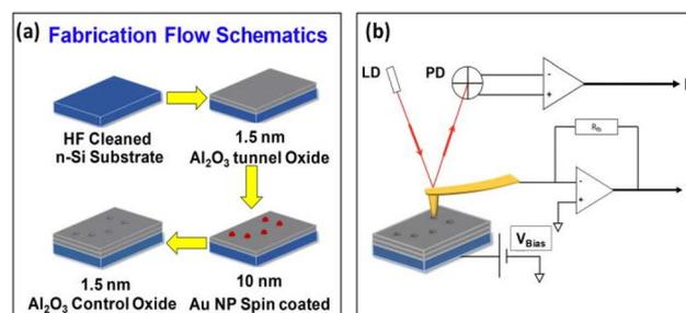
Fig. 9 (a) Fabrication process for nanomemory devices and (b) the circuit setup for probing a single Au-NP using conductive atomic force microscopy (C-AFM). Reproduced from ref. 47 with permission from [AIP Publishing], copyright [2020].
