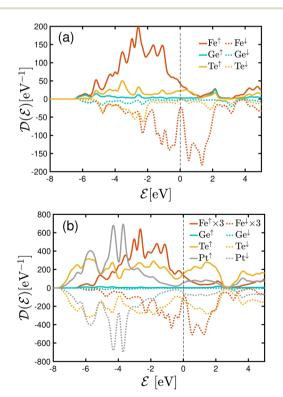
Fig. 2 DOS plots for (a) the freestanding monolayer F4GT and (b) the F4GT sandwiched between two layers of PtTe2.
