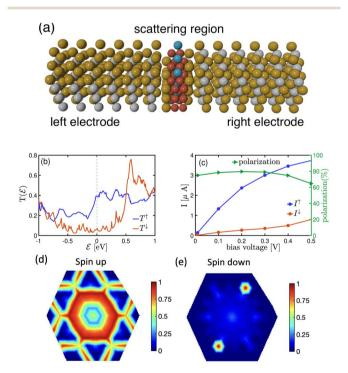
(a) Schematic representation of a two-probe model for NEGF calculations, depicting a monolayer F4GT sandwiched between two PtTe<sub>2</sub> electrodes. (b) The transmission spectrum of the system under zero bias voltage. (c) Variation of spin polarization, spin-up current  $(I\uparrow)$ and spin-down current ( $I\downarrow$ ) with bias voltage. The  $k_{\parallel}$ -resolved transmission probability for (d) spin-up and (e) spin-down electrons at the Fermi energy in the absence of bias voltage.
