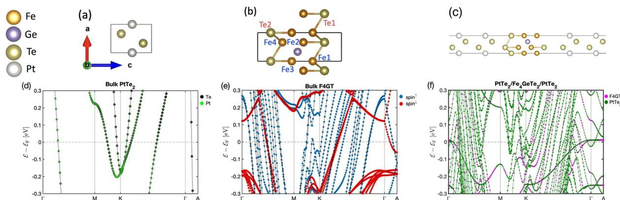
Fig. 1 The atomic structures of (a) PtTe<sub>2</sub>, (b) F4GT, and (c) F4GT sandwiched between two PtTe<sub>2</sub> electrodes. Panels (d–f) showcase the corresponding electronic band structures without considering spin–orbit coupling: (d) atom-projected electronic band structure for bulk PtTe<sub>2</sub>, (e) spin-projected electronic band structure for bulk F4GT, and (f) layer-projected electronic band structure for monolayer F4GT sandwiched between two PtTe<sub>2</sub> electrodes.
