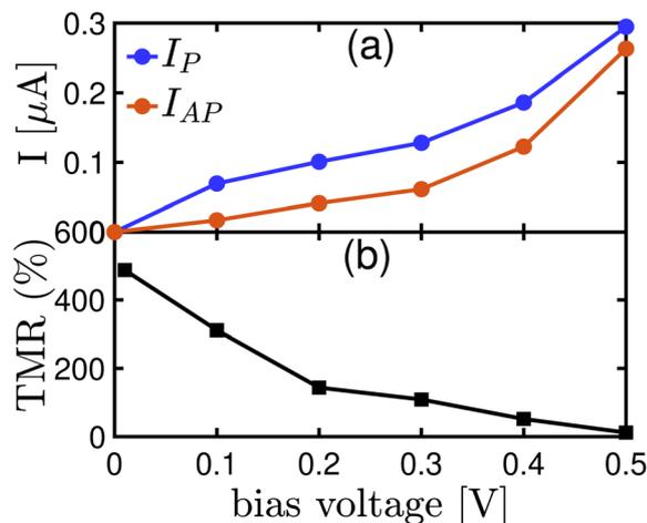
Fig. 10 (a) Total current, a summation of both spin-up and spin-down currents, of  $\text{Fe}_4\text{GeTe}_2/\text{monolayer GaTe}/\text{Fe}_4\text{GeTe}_2$  magnetic tunnel junction sandwiched between two  $\text{PtTe}_2$  electrodes at the parallel and antiparallel state as a function of bias voltage. (b) Variation of the TMR with bias voltage for the same MTJ.
