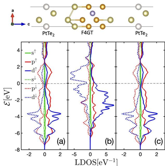
Fig. 5 Orbital-projected local density of states for (a) the left electrode's PtTe<sub>2</sub> layer interfacing with F4GT, (b) F4GT itself, and (c) the right electrode's PtTe<sub>2</sub> layer interfacing with F4GT.
