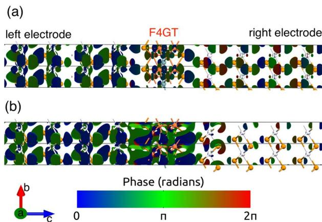
Fig. 4 The isosurface plots of transmission eigenstates for a monolayer F4GT placed between two PtTe<sub>2</sub> electrodes under zero bias voltage at the Fermi level for (a) the spin-up and (b) the spin-down channel. For both channels, the isosurface values are fixed at  $0.17 \text{ \AA}^{-3} \text{ eV}^{-1}$ .
