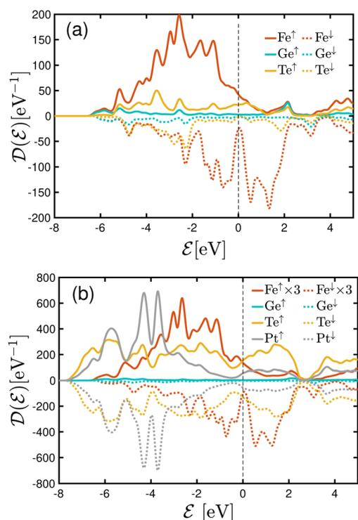
Fig. 2 DOS plots for (a) the freestanding monolayer F4GT and (b) the F4GT sandwiched between two layers of PtTe<sub>2</sub>.
