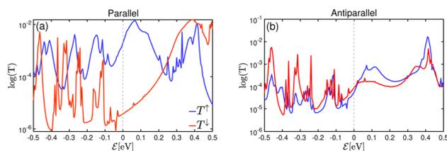
Fig. 9 Transmission characteristics of the Fe<sub>4</sub>GeTe<sub>2</sub>/bilayer GaTe/Fe<sub>4</sub>GeTe<sub>2</sub> in the (b) parallel and (b) antiparallel state under zero bias voltage on a logarithmic scale.
