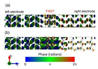
Fig. 4 The isosurface plots of transmission eigenstates for a monolayer F4GT placed between two PtTe $_2$  electrodes under zero bias voltage at the Fermi level for (a) the spin-up and (b) the spin-down channel. For both channels, the isosurface values are fixed at 0.17 Å $^{-3}$  eV $^{-1}$ .
