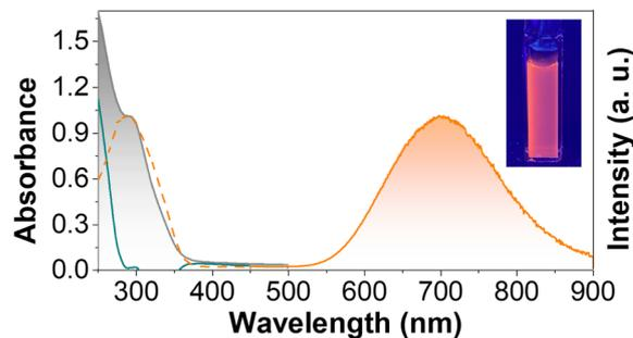
Fig. 2 Absorption spectrum of AuNC@NAC (grey area) in aqueous solution; the excitation spectrum at  $\lambda_{\text{em}} = 700$  nm (orange dashed line) normalized at the absorption shoulder at 295 nm; the difference spectrum between AuNC@NAC absorption and AuNC excitation (dark cyan line); and the PL spectrum (orange area) at  $\lambda_{\text{exc}} = 310$  nm of AuNC@NAC.
