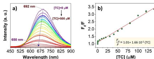
Fig. 6 (a) PL spectra of AuNC@NAC upon addition of [TC] from 0 to  $500\text{ }\mu\text{M}$ . (b) Relationship between the relative PL intensity  $F_0/F$  and the concentration of TC in the range  $0.1\text{--}140\text{ }\mu\text{M}$ , where  $F_0$  represents the PL intensity in the absence of TC and  $F$  represents the PL intensity in the presence of TC.
