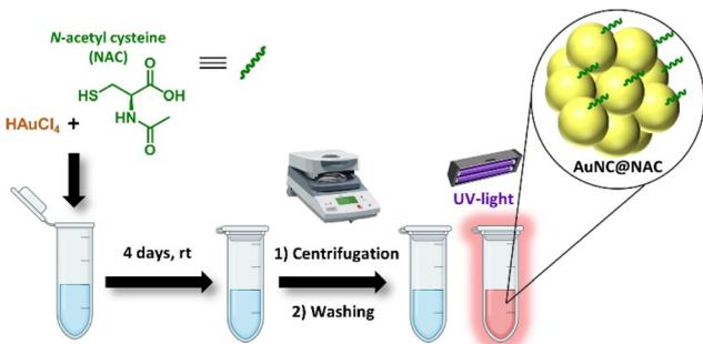
Fig. 1 Schematic representation of the synthesis of AuNC@NAC.
