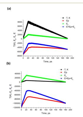
Fig. 7 Calculated temperature and NP energies vs. time for  $T_{\rm max}=8000$  K. Here, simulations are performed for a single Au NP with radius (a) R=20 uc, and (b) R=50 uc. Energy units are cal mol<sup>-1</sup>.
