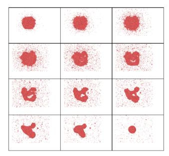
Fig. 5 Snapshots obtained in MD simulations showing the time evolution of Au nanocluster with radius R = 50 uc (uc is unit cells length, 0.407 nm for Au),  $N = 30\,845$  atoms and maximum temperature  $T_{\text{max}} = 8000 \text{ K}$  obtained at time delays t = 0.1, 5, 10 ps (first row), 20, 30, 40 ps, (second row), 50, 60, 70 ps (third row), 80, 100, 150 ps (bottom row) after the beginning of strong and short (20 ps) heating (from left to right)
