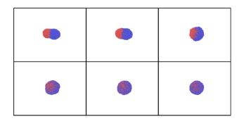
Fig. 11 Snapshots obtained in the heating of Janus AuNi nanoparticles (6125 atoms, where 3061 atom of Au and 3064 of Ni) with heating shown in Fig. 3S.†  $T_{\text{max}} = 2700 \text{ K}$ , time delays are 0, 10, 20 ps (upper row), 50, 70, and 90 ps (bottom row), from left to right.
