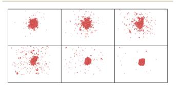
Fig. 4 Snapshots from MD simulations showing the time evolution of Au nanocluster with radius R=20 uc (1 uc = 4.07 Å for Au), N=1959atoms, and maximum temperature  $T_{\rm max} = 8000$  K obtained at t = 0.1, 5, 10 ps (upper row), 20, 50, 100 ps (bottom row) from left to right.
