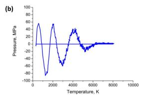
Fig. 8 Calculated pressure–temperature dependencies (a) for Au nanoparticle with radius  $R=20~\rm uc$ ; (b) – the same for radius  $R=50~\rm uc$ . The heating–cooling conditions are the same as in Fig. 4–7.
