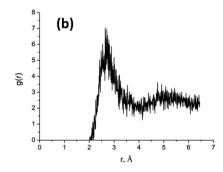
Fig. 6 Calculated radial distribution function (RDF) for Au cluster with R=20 uc, (a) at t=0.1 ps and (b) – the same at t=10 ps.
