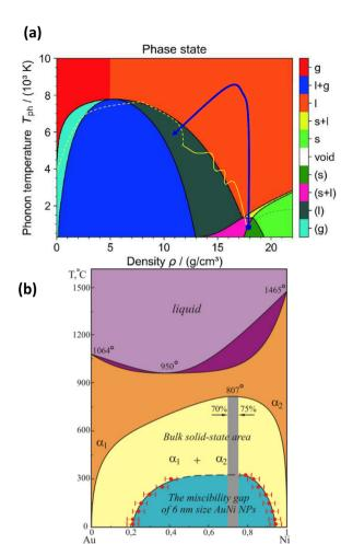
Fig. 2 (a) – Temperature–density phase diagram of gold with phase states:  $^{61}$  s—solid; l—liquid; g—gas; l + g—liquid–gas mixture; s + l—melting; (s)—metastable solid; (s + l)—metastable melting; (l)—metastable liquid; (g)—metastable gas. bn and sp are binodal and spinodal curves, respectively. (b) – Binary Au–Ni phase diagram.  $^{63-65}$
