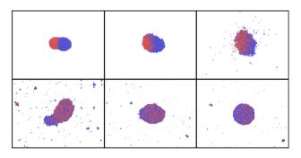
Fig. 14 Simulation snapshots for AuNi Janus NP and  $T_{\rm max}$  = 8000 K, at time t = 10, 20, 30, 50, 70, 90 ps.
