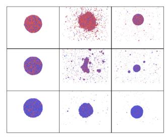
Fig. 9 Snapshots obtained in MD simulations for AuNi nanoparticle ( $R\sim40~\rm uc$ ,  $N\sim15~820~\rm atoms$ ) heated up to 9000 K and cooled down to 300 K, showing the role of composition for time delays of 0, 50, and 160 ps for three Ni fractions (top - 20%, middle row - 50%, bottom - 80%).
