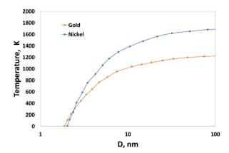
Fig. 1 Size-dependent melting temperature of gold and nickel nanoparticles.<sup>59,60</sup>
