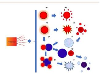
Fig. 3 Schematics of nanoparticle transformations under fast heating: (a) and (b) – evaporation, (c) and (d) – fragmentation, (d) and (e) sintering, (e) and (f) and (d)–(f) – alloying, (e)–(h) aggregation, (h) and (f) – fragmentation of an aggregate.
