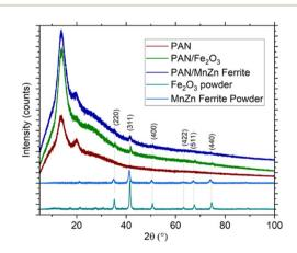
Fig. 3 XRD spectra of the PAN, PAN/Fe<sub>2</sub>O<sub>3</sub> and PAN/MnZn ferrite using Co Kα radiation. XRD of the nanoparticles is also provided.
