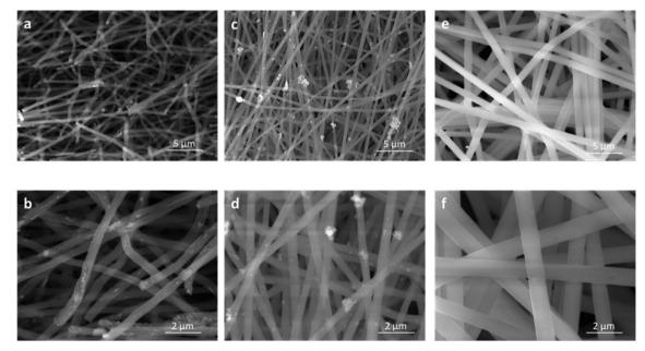
Fig. 11 Post-DMA examination of the (a and b) PAN/Fe<sub>2</sub>O<sub>3</sub>, (c and d) PAN/MnZn ferrite, and (e and f) PAN at 20k× and 50k×.
