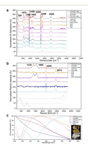
Fig. 4 (a) FTIR (top), (b) Raman (middle) and (c) UV-vis (bottom) spectra of the different PAN membranes and nanoparticles normalized to the highest peak (1446 and 2245 cm $^{-1}$  for IR and Raman, respectively). Insert in UV-vis showing a visual representation of membranes before (fibrous) and after (film) laser irradiation – bottom PAN, middle PAN with ferrite (represented as FeO), top PAN with MnZn ferrite (represented as MxO).
