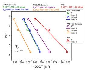
Fig. 9 Comparison of slopes yielding activation energy of the samples measured from the  $T_{\rm g1}$  from E''.
