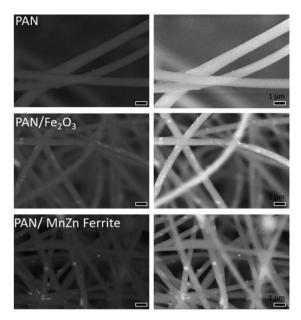
Fig. 5 HRSEM imaging in BSE (left) and SE (right) modes for three nanofiber types.
