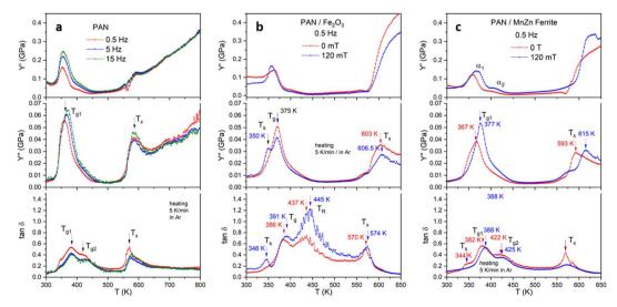
Fig. 8 DMA of the (a) PAN sample at three different frequencies without applied external field (0 T), comparison of the PAN/Fe<sub>2</sub>O<sub>3</sub> and PAN/MnZn ferrite samples at (b) 0 T and (c) 120 mT and 0.5 Hz frequency. (Top) Storage modulus, (middle) loss modulus, and (bottom) tan  $\delta$ .
