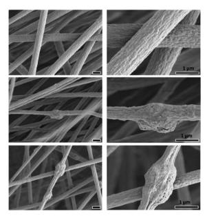
Fig. 6 The surface texture of the PAN (top), PAN/Fe<sub>2</sub>O<sub>3</sub> (middle) and PAN/MnZn ferrite (bottom) nanofibers
