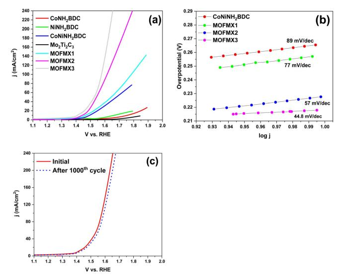
Electrocatalytic OER efficiency (a) LSV curves, (b) Tafel slope, (c) LSV curves of MOFMX3 before and after 1000 CV cycles.
