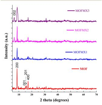
Fig. 1 XRD patterns of CoNiNH<sub>2</sub>BDC MOF and MOFMX composites.
