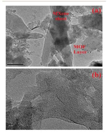
Fig. 3 TEM images of MOFMX3 composite (scale bar (a) 50 and (b) 20 nm).
