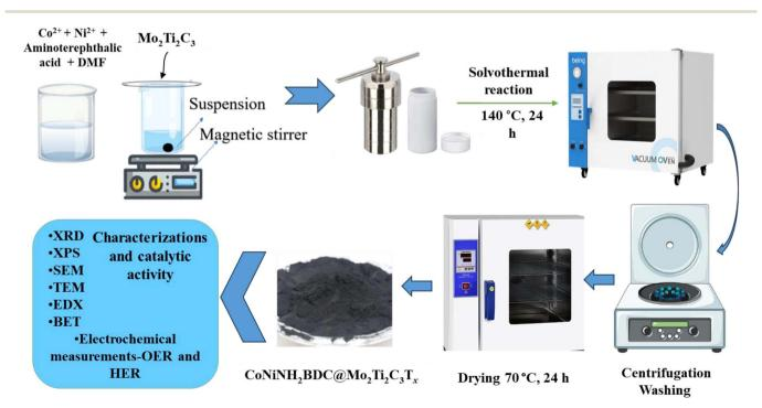
Scheme 1 Schematic diagram for the synthesis of CoNiNH<sub>2</sub>BDC@Mo<sub>2</sub>Ti<sub>2</sub>C<sub>3</sub>T<sub>x</sub>.
