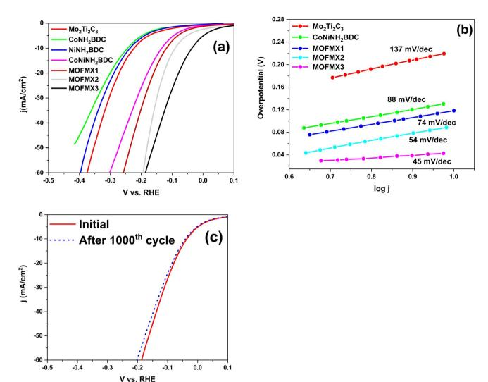
Fig. 7 Electrocatalytic HER efficiency (a) LSV curves, (b) Tafel slope, and (c) LSV curves of MOFMX3 before and after 1000 CV cycles.
