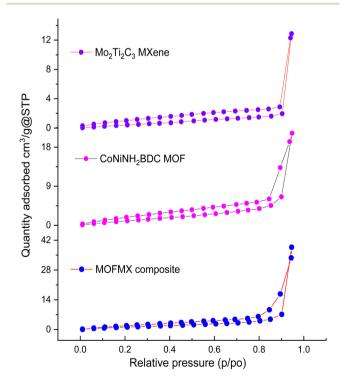
Fig. 5  $N_2$  adsorption/desorption isotherm of  $Mo_2Ti_2C_3$  MXene,  $CoNiNH_2BDC$  MOF and MOFMX3 composites.
