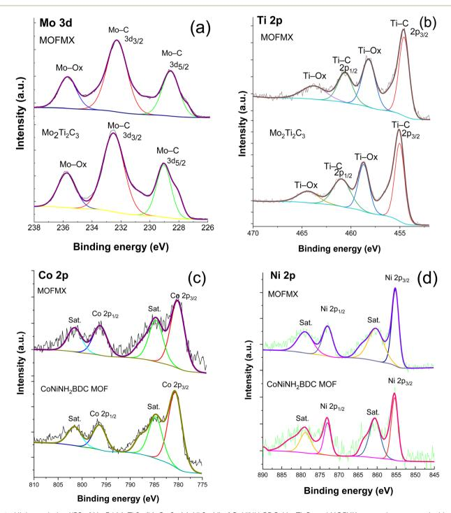
Fig. 4 High-resolution XPS of Mo 3d (a), Ti 2p (b), Co 2p (c), Ni 2p (d) of CoNiNH<sub>2</sub>BDC, Mo<sub>2</sub>Ti<sub>2</sub>C<sub>3</sub> and MOFMX composite compared with each other.
