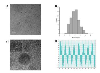
Fig. 2 Characterization of RCL-CDs. (A) Transmission electron microscopy (TEM) images of *Rubia cordifolia* L.-carbon dots (RCL-CDs) displaying ultra-small particles. (B) Histogram depicting particle size distribution. (C) High-resolution TEM (HRTEM) image of RCL-CDs. (D) The inset shows a HRTEM image of atomic lattice fringes.
