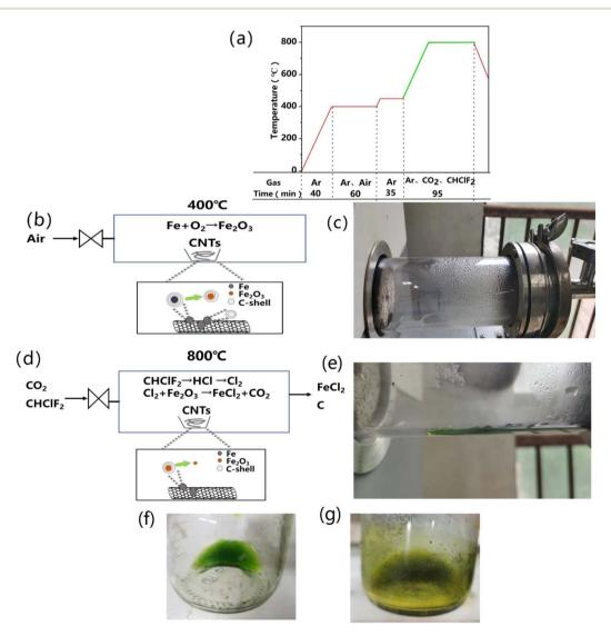
Fig. 3 (a) Diagram of the Freon-CO<sub>2</sub>-assisted purification process. (b) Schematic of air pre-oxidation. (c) Moisture condensed at the end of the tube furnace. (d) Schematic of the Freon-CO<sub>2</sub>-assisted purification process. (e) Liquid FeCl<sub>2</sub> at the end of the tube furnace. (f) Fresh liquid collected after the purification, and (g) liquid stayed in air for 48 h.
