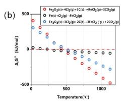
Fig. 2 (a) Melting and boiling points of substances related to the elements Fe, Co, and Ni. (b) Standard Gibbs free energy changes for reactions associated with Fe in purification processes of the SWCNTs.
