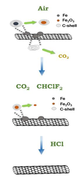
Fig. 1 Schematic of the Freon– ${\rm CO_2}$ -assisted purification process of SWCNTs.
