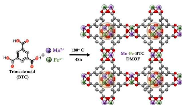
Fig. 1 Dual metal-organic framework as electrode for LMBs.
