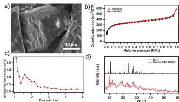
Fig. 2 (a) SEM image of Mn-Fe-BTC DMOF, (b) N<sub>2</sub> isotherm adsorption/desorption isotherm analysis of Mn-Fe-BTC DMOF, (c) pore size distribution of Mn-Fe-BTC DMOF and (d) PXRD spectra of BTC (black) and Mn-Fe-BTC DMOF (red).
