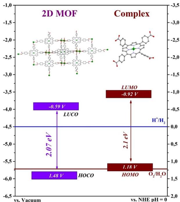
Scheme 2 Structures and band alignment of the 2D  $\text{Cu}_2(\text{CuTCPP})$  MOF (left) and the Cu TCPP molecular complex (right) referred to the NHE at pH 0 and vs. vacuum. The blue line indicates the  $\text{H}^+/\text{H}_2$  reduction potential and red line indicates  $\text{O}_2/\text{H}_2\text{O}$  oxidation potential.
