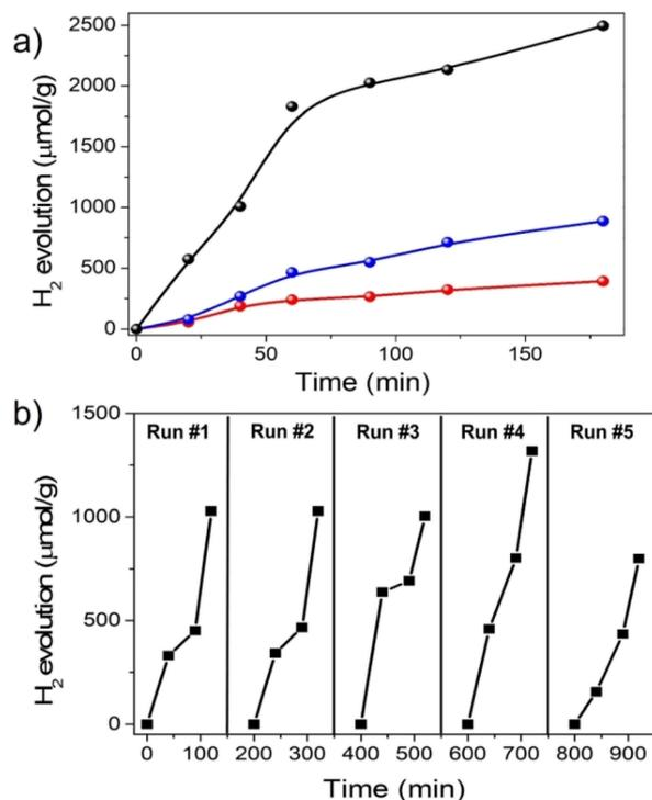
Fig. 3 (a) Temporal profile of H<sub>2</sub> evolution using Cu<sub>2</sub>(CuTCPP) (black), CuTCPP molecular complex (red) and Cu<sub>2</sub>(FeTCPP) (blue) dispersions at 1 mg mL<sup>-1</sup> in H<sub>2</sub>O : MeOH mixtures (70 : 30, v : v) under 1080 mW cm<sup>-2</sup> illumination from a Xe lamp using a 450 nm cut-off filter. (b) H<sub>2</sub> evolution from five consecutive uses of the Cu<sub>2</sub>(CuTCPP) photocatalyst for 2 h.
