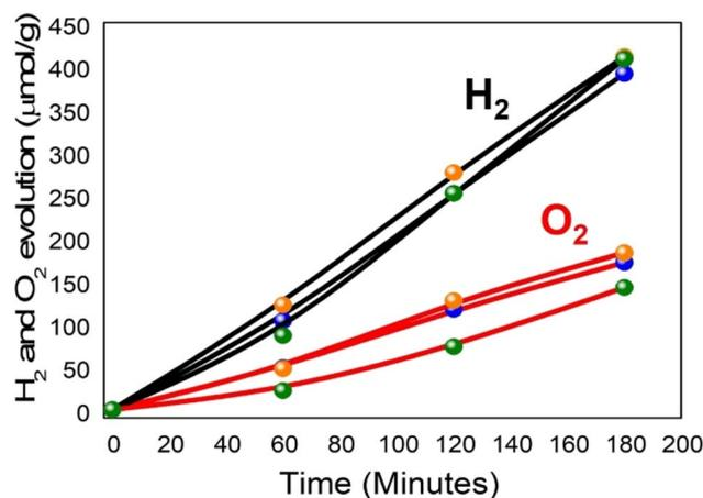
Fig. 4 Temporal profile of H<sub>2</sub> (black lines) and O<sub>2</sub> (red lines) evolution of three consecutive uses of a Cu<sub>2</sub>(CuTCPP) dispersion at 1 mg mL<sup>-1</sup> in pure water under visible light at 1080 mW cm<sup>-2</sup> illumination from a Xe lamp using a 450 nm cut-off filter.
