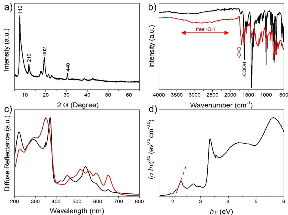
**Fig. 1** (a) XRD pattern of  $\text{Cu}_2(\text{CuTCPP})$ , (b) FTIR spectra of  $\text{H}_2\text{TCPP}$  (red) and  $\text{Cu}_2(\text{CuTCPP})$  (black), (c) diffuse reflectance UV-vis spectra of  $\text{H}_2\text{TCPP}$  (red) and  $\text{Cu}_2(\text{CuTCPP})$  (black) and (d) Tauc plot obtained from the  $\text{Cu}_2(\text{CuTCPP})$  diffuse reflectance spectrum. The dashed line indicates the intersection used to calculate the optical band gap.
