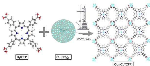
Scheme 1 Preparation procedure of Cu<sub>2</sub>(CuTCPP).
