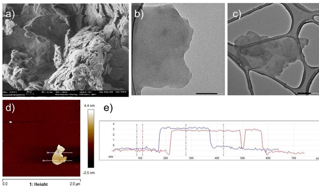
**Fig. 2** FESEM image of  $\text{Cu}_2(\text{CuTCPP})$  (scale bar 300 nm) (a). TEM images of  $\text{Cu}_2(\text{CuTCPP})$  (b) and (c). Scale bars are 100 nm and 200 nm, in (b) and (c), respectively. The AFM image of  $\text{Cu}_2(\text{CuTCPP})$  (d). Cross section measurements (e) of the  $\text{Cu}_2(\text{CuTCPP})$  sheet presented in panel (d).
