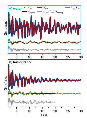
Fig. 5 Neutron PDF (nPDF) and refinements using the  $CoFe_2O_4$  spinel structure in space-group  $Fd\overline{3}m$ . (A) Refinement of the nPDF of the water-synthesized nanoparticles. Here the magnetic PDF is furthermore refined as the difference curve using a collinear model. (B) Refinement of the nPDF of the tert-butanol-synthesized nanoparticles.
