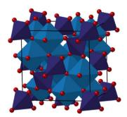
Fig. 1 Structural representation of a normal spinel in the space group  $Fd\bar{3}m$ ,<sup>24</sup> where  $M_{Oh}$  cations are shown in blue, while  $M_{Td}$  cations are shown in purple (M = Co/Fe). Oxygens are represented in red.
