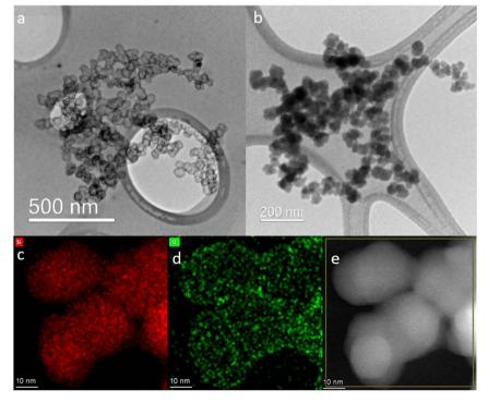
Fig. 3 TEM images of thermally oxidized cCVD Si nanoparticles at 300 °C (a) and 500 °C (b) treated in pH 9.0. HSSs are seen for the 300 °C heat treated nanoparticles, while the 500 °C heat treated nanoparticles are solid. EDS mapping (bottom panel) of the 500 °C treated cCVD Si sample after base treatment (pH 9.0). The distribution of silicon ((c) red) and oxygen ((d) green) and the dark field TEM image of the mapped region (e).
