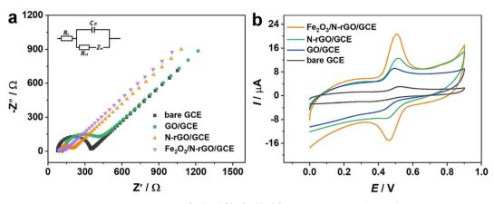
Fig. 3 (a) Nyquist plots of different electrodes in 10 mM  $K_3$ [Fe(CN)<sub>6</sub>]  $K_4$ [Fe(CN)<sub>6</sub>] solution including 0.1 M KCl. Inset: the equivalent circuit. (b) CVs of different electrodes in 0.1 M PBS with a pH value of 3.0 containing 100  $\mu$ M rutin.
