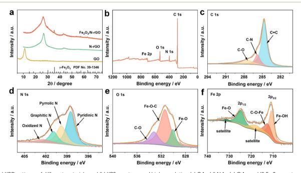
Fig. 2 (a) XRD patterns of different materials, and (b) XPS spectrum and high-resolution (c) C 1s, (d) N 1s, (e) O 1s, and (f) Fe 2p spectra of  $Fe_2O_3/N-rGO$ .
