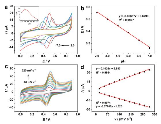
Fig. 4 (a) CV curves of 100  $\mu$ M rutin on Fe<sub>2</sub>O<sub>3</sub>/-N-rGO/GCE at different pH, and (b) the relationship between pH values and potential. (c) CV curves of 100  $\mu$ M rutin at different scan rates. (d) The corresponding relationship between currents (*I*) and scan rates (v).
