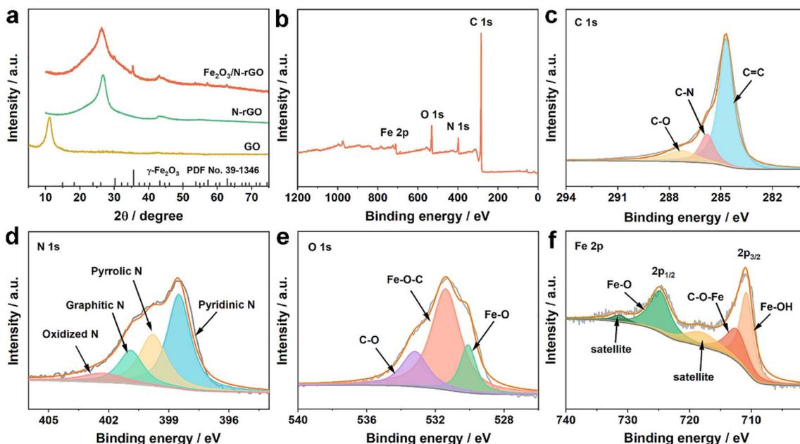
Fig. 2 (a) XRD patterns of different materials, and (b) XPS spectrum and high-resolution (c) C 1s, (d) N 1s, (e) O 1s, and (f) Fe 2p spectra of Fe<sub>2</sub>O<sub>3</sub>/N-rGO.
