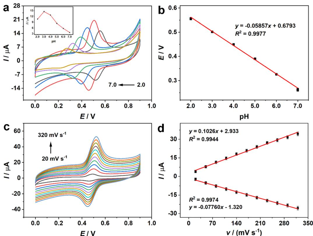
Fig. 4 (a) CV curves of 100 μM rutin on Fe<sub>2</sub>O<sub>3</sub>/N-rGO/GCE at different pH, and (b) the relationship between pH values and potential. (c) CV curves of 100 μM rutin at different scan rates. (d) The corresponding relationship between currents ( $I$ ) and scan rates ( $v$ ).
