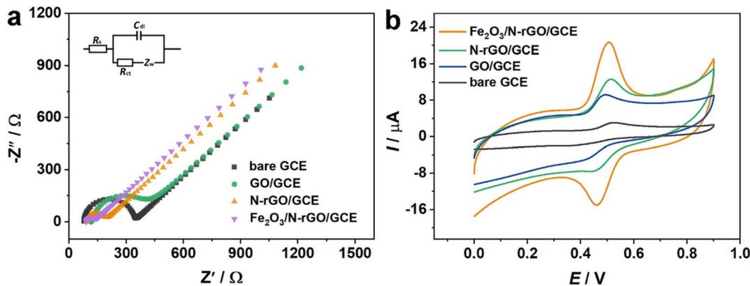
Fig. 3 (a) Nyquist plots of different electrodes in 10 mM  $K_3[Fe(CN)_6]/K_4[Fe(CN)_6]$  solution including 0.1 M KCl. Inset: the equivalent circuit. (b) CVs of different electrodes in 0.1 M PBS with a pH value of 3.0 containing 100  $\mu$ M rutin.
