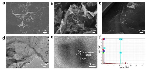
Fig. 1 SEM images of (a) GO, (b) N-rGO, (c) Fe<sub>2</sub>O<sub>3</sub>/N-rGO, (d and e) TEM and HRTEM images of Fe<sub>2</sub>O<sub>3</sub>/N-rGO, and (f) EDX result of Fe<sub>2</sub>O<sub>3</sub>/N-rGO.
