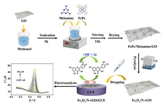
Scheme 1 Synthesis of Fe<sub>2</sub>O<sub>3</sub>/N-rGO and the sensing process of rutin.
