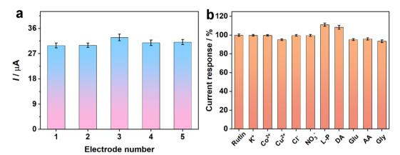
Fig. 6 (a) Reproducibility for the five independently prepared electrodes towards 100  $\mu$ M rutin. (b) Selectivity of the proposed sensor for 1000  $\mu$ M K<sup>+</sup>, Co<sup>2+</sup>, Cu<sup>2+</sup>, Cl<sup>-</sup>, and NO<sub>3</sub><sup>-</sup> and 100  $\mu$ M  $_{L}$ -P, DA, Glu, AA, and Gly for the detection of 10  $\mu$ M rutin.
