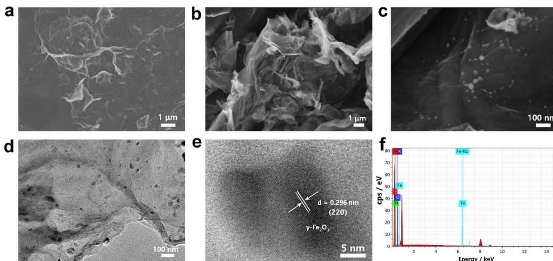
Fig. 1 SEM images of (a) GO, (b) N-rGO, (c)  $\text{Fe}_2\text{O}_3/\text{N-rGO}$ , (d and e) TEM and HRTEM images of  $\text{Fe}_2\text{O}_3/\text{N-rGO}$ , and (f) EDX result of  $\text{Fe}_2\text{O}_3/\text{N-rGO}$ .
