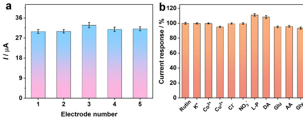
Fig. 6 (a) Reproducibility for the five independently prepared electrodes towards 100  $\mu\text{M}$  rutin. (b) Selectivity of the proposed sensor for 1000  $\mu\text{M}$   $\text{K}^+$ ,  $\text{Co}^{2+}$ ,  $\text{Cu}^{2+}$ ,  $\text{Cl}^-$ , and  $\text{NO}_3^-$  and 100  $\mu\text{M}$  L-P, DA, Glu, AA, and Gly for the detection of 10  $\mu\text{M}$  rutin.
