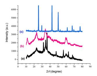
Fig. 5 X-ray diffraction of the catalyst and its intermediates, (a) layered LDH@PTRMS, double hydroxide, (b) and (c) LDH@PTRMS@DCMBA@Cul.
