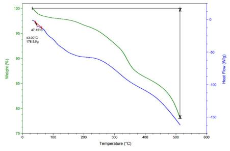
Fig. 4 TGA and DSC thermal analyses of the LDH@PTRMS@DCMBA@Cul catalyst.
