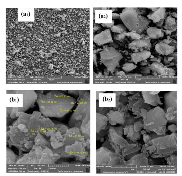
Fig. 3 FESEM images of ( $a_1$  and  $a_2$ ) LDH@PTRMS and ( $b_1$  and  $b_2$ ) LDH@PTRMS@DCMBA@Cul catalyst.
