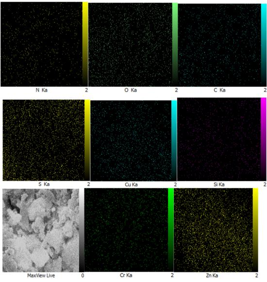
Fig. 7 Elemental mapping analysis (MAPPING) of the LDH@PTRMS@DCMBA@Cul catalyst.
