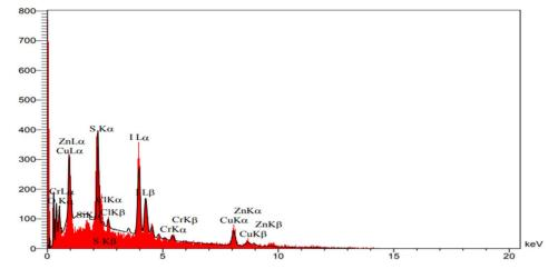
Fig. 6 EDX analysis of the LDH@PTRMS@DCMBA@Cul catalyst.
