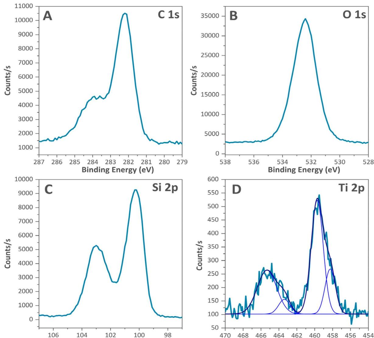
Fig. 3 XPS spectra of Ti-grafted SiC supports "TiO<sub>2</sub>@SiC/SiO<sub>2</sub>-p". (A: C1s, B: O1s, C: Si2p, D: Ti 2p).
