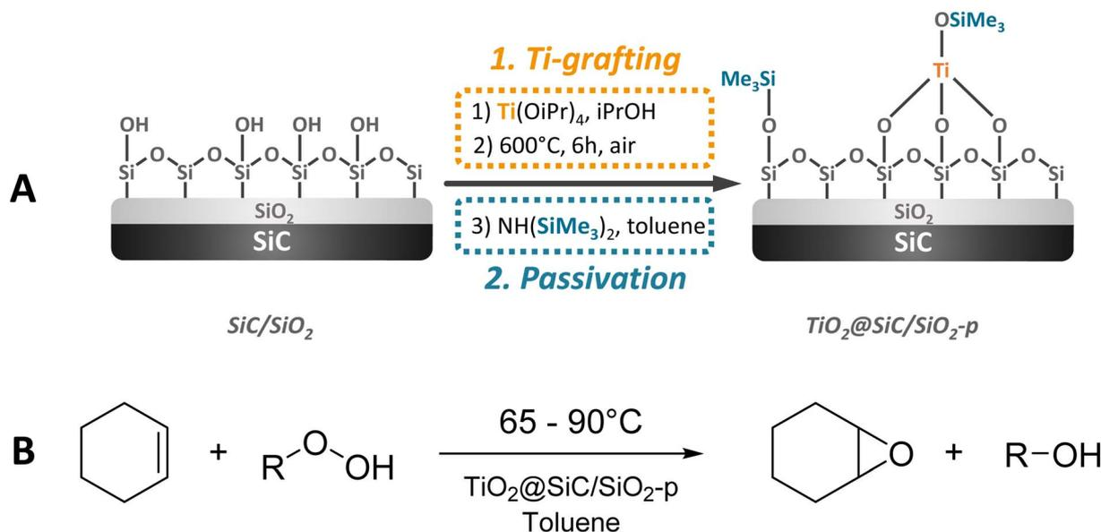
Scheme 1 (A) Synthesis protocol for the formation of the SiC-based  $\text{TiO}_2$  catalyst. (B) Epoxidation reaction of cyclohexene.
