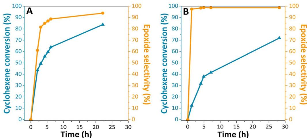
Fig. 4 Conversion of cyclohexene (blue) and epoxide selectivity (yellow) results from catalytic tests of the  $\text{TiO}_2@\text{SiC}/\text{SiO}_2\text{-p}$  catalyst with (A) *tert*-butyl hydroperoxide and (B) cumene hydroperoxide as the oxidant.
