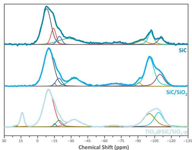
Fig. 2  $^{29}\text{Si}$  CP-MAS solid-state NMR spectra of the SiC, SiC/SiO<sub>2</sub> and  $\text{TiO}_2@\text{SiC}/\text{SiO}_2$  materials (top to bottom).
