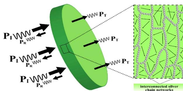
Fig. 12 Schematic EMI shielding mechanism for the PLA/Ag composites with novel segregated electrically conductive Ag networks. Reprinted with permission. Copyright (2018).<sup>173</sup>
