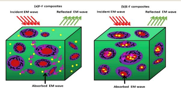
Fig. 11 Cartoon illustrating the EMI shielding mechanism for the composites (a) F-F composites [PVDF $-Fe_3O_4$ ], (b) E-F composites [HDPE $-Fe_3O_4$ ], (b) E-F composites [HDPE $-Fe_3O_4$ ], (c) E-F composites (a) E-F composites (b) E-F composites (c) E-F composites (b) E-F composites (c) Fe<sub>3</sub>O<sub>4</sub>]. Reprinted with permission. Copyright (2018). 165
