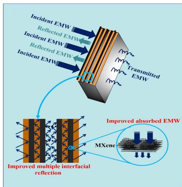
Fig. 6 Schematic of electromagnetic microwave dissipation in the PVA/MXene multilayered films. Reprinted with permission. Copyright (2020).<sup>78</sup>
