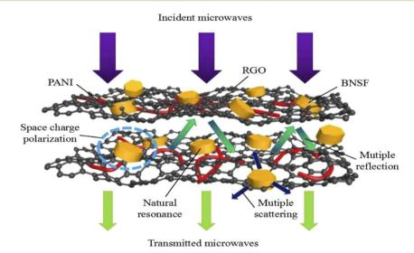
Fig. 8 Schematic representation of the microwave attenuation mechanism in RGO/PANI/BNSF nanocomposites. Reprinted with permission. Copyright (2019).109
