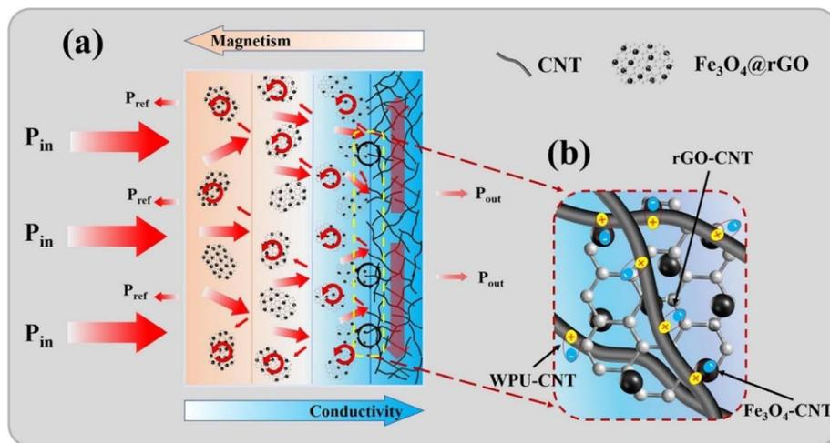
Fig. 7 (a) EMI shielding mechanism of the  $Fe_3O_4@rGO/MWCNT/WPU$  composite. (b) Polarization relaxation loss mechanism of the interface between  $Fe_3O_4@rGO/WPU$  and  $MWCNT/WPU$ . Reprinted with permission. Copyright (2020).<sup>99</sup>
