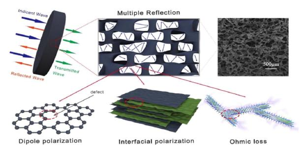
Fig. 9 Possible electromagnetic shielding mechanism of the  $Ti_3C_2T_x/RGO/ANFs$  hybrid aerogel. Reprinted with permission. Copyright (2022). 128
