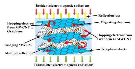
Fig. 3 Schematic representation of the proposed EMI shielding mechanism in PUGCNT nanocomposites. Reprinted with permission. Copyright (2017).<sup>40</sup>
