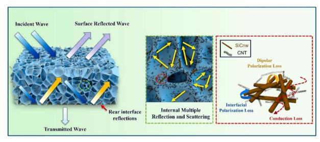
Fig. 10 Schematic illustration of EM wave dissipation in the PVDF/CNT/SiCnw composite foams. Reprinted with permission. Copyright (2023). 140
