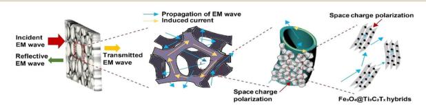
Fig. 13 Schematic diagram of the EM waves absorption in the  $Fe_3O_4@Ti_3C_2T_x/GF/PDMS$  composite. Reprinted with permission. Copyright (2020). 186
