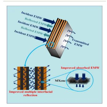
Fig. 6 Schematic of electromagnetic microwave dissipation in the PVA/MXene multilayered films. Reprinted with permission. Copyright (2020).78
