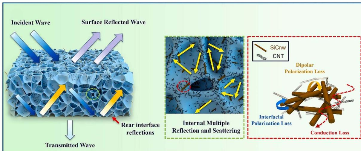
Fig. 10 Schematic illustration of EM wave dissipation in the PVDF/CNT/SiCnw composite foams. Reprinted with permission. Copyright (2023).<sup>140</sup>
