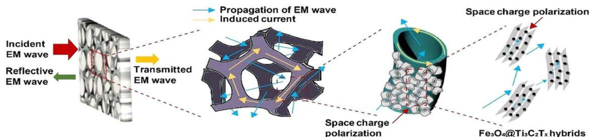
Fig. 13 Schematic diagram of the EM waves absorption in the  $Fe_3O_4@Ti_3C_2T_x/GF/PDMS$  composite. Reprinted with permission. Copyright (2020).<sup>186</sup>
