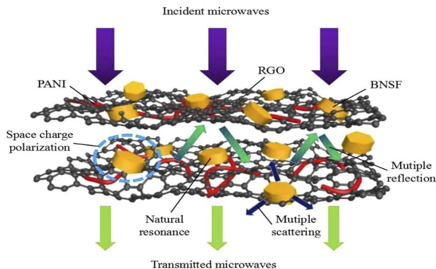
Fig. 8 Schematic representation of the microwave attenuation mechanism in RGO/PANI/BNSF nanocomposites. Reprinted with permission. Copyright (2019).<sup>109</sup>
