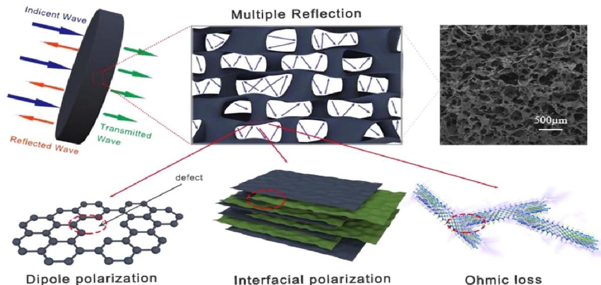
Fig. 9 Possible electromagnetic shielding mechanism of the  $\text{Ti}_3\text{C}_2\text{T}_x/\text{RGO}/\text{ANFs}$  hybrid aerogel. Reprinted with permission. Copyright (2022).<sup>128</sup>
