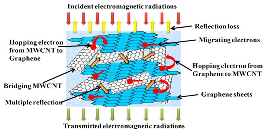
Fig. 3 Schematic representation of the proposed EMI shielding mechanism in PUGCNT nanocomposites. Reprinted with permission. Copyright (2017).<sup>40</sup>
