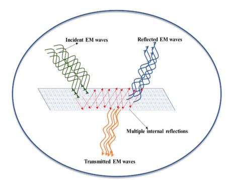
Fig. 2 Pictorial depiction of the mechanism of an EMI shielding material.
