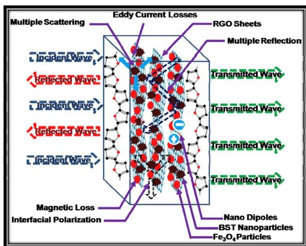
Fig. 5 Schematic representation of a possible mechanism of EMI shielding in the PBRF composite. Reprinted with permission. Copyright (2018).<sup>76</sup>
