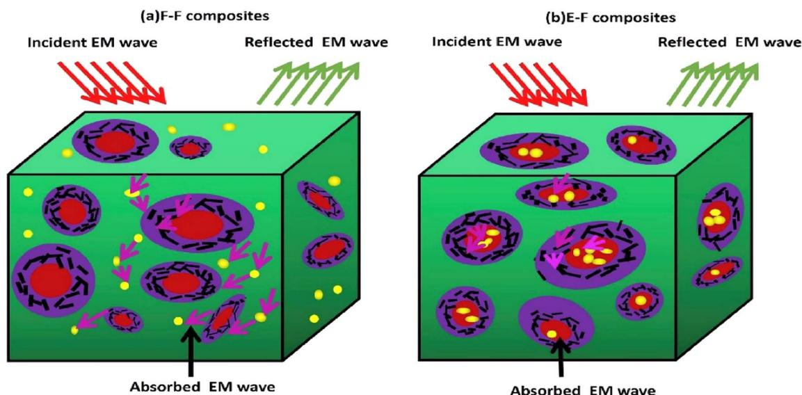
Fig. 11 Cartoon illustrating the EMI shielding mechanism for the composites (a) F–F composites [PVDF– $\text{Fe}_3\text{O}_4$ ], (b) E–F composites [HDPE– $\text{Fe}_3\text{O}_4$ ]. Reprinted with permission. Copyright (2018).<sup>165</sup>
