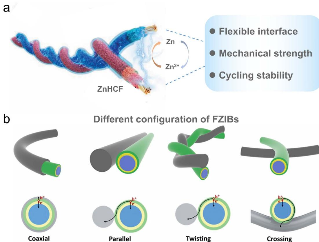
Fig. 3 (a) Schematic diagram of the energy storage mechanism of FZIBs, highlighting the key factors influencing their practical application. Reproduced from ref. 59 with permission from Elsevier, copyright 2024. (b) Different structural forms of FZIBs and their charge transfer pathways. Reproduced with permission from ref. 60. Copyright 2022 American Chemical Society.
