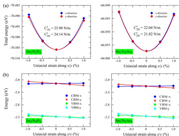
Fig. 8 Total energy  $E_{\text{tot}}(\epsilon_{\text{uni}})$  (a) and band edge alignment  $\Delta E_{\text{edge}}$  (b) as functions of uniaxial strains  $\epsilon_{\text{uni}}$  along  $x$ - and  $y$ -directions.
