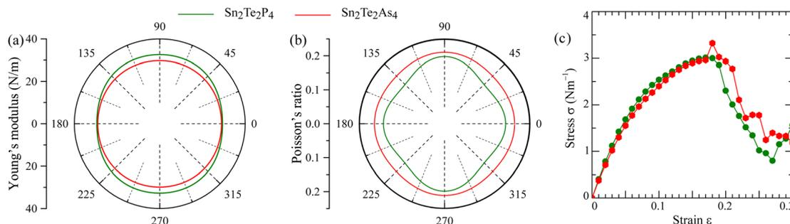
Fig. 2 Mechanical properties of  $\text{Sn}_2\text{Te}_2\text{P}_4$  (green lines) and  $\text{Sn}_2\text{Te}_2\text{As}_4$  (red lines) monolayers including (a) Young's modulus and (b) Poisson's ratio as angular functions and (c) dependence of stress ( $\sigma$ ) on strain ( $\epsilon$ ).
