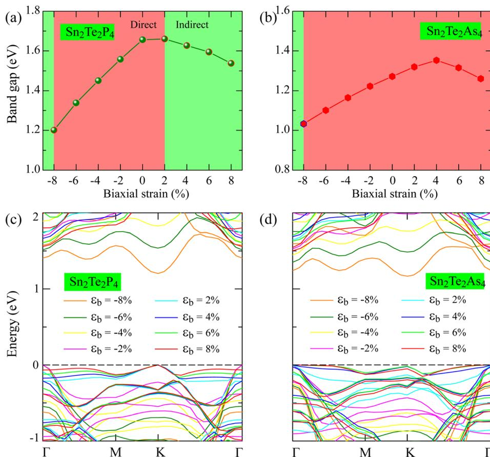
Fig. 4 Variation in the band gap and band structure of (a and c)  $\text{Sn}_2\text{Te}_2\text{P}_4$  and (b and d)  $\text{Sn}_2\text{Te}_2\text{As}_4$  monolayers subjected to strains ranging from  $-8\%$  to  $8\%$ .
