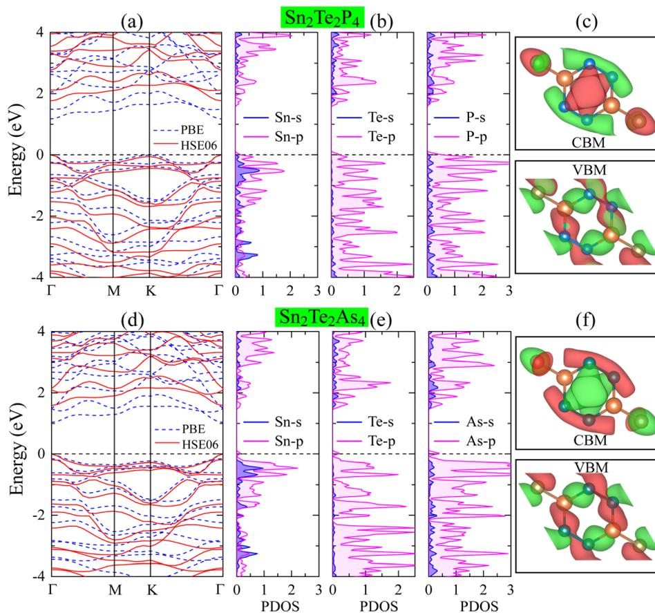
Fig. 3 Electronic characteristics of the (a)–(c)  $\text{Sn}_2\text{Te}_2\text{P}_4$  monolayer and (d)–(f)  $\text{Sn}_2\text{Te}_2\text{As}_4$  monolayers: band structure calculated by PBE (blue dashed lines) and HSE06 (red solid lines) methods; partial density of states PDOS and charge density iso-surfaces of the VBM and CBM with an iso-surface value of  $0.02 e \text{ \AA}^{-6}$ ; both were calculated by the HSE06 method.
