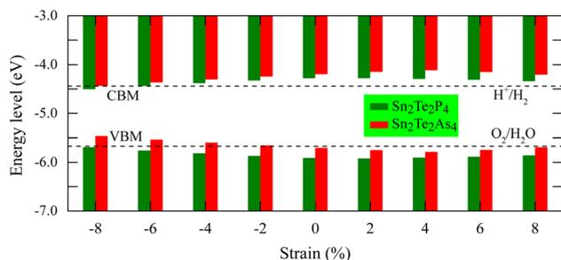
Fig. 7 The VBM and CBM positions of  $\text{Sn}_2\text{Te}_2\text{P}_4$  (green) and  $\text{Sn}_2\text{Te}_2\text{As}_4$  (red) in relation to water redox potentials at the normal hydrogen electrode (NHE) and vacuum level. The reduction potential of  $\text{H}^+/\text{H}_2$  and the oxidation potential of  $\text{O}_2/\text{H}_2\text{O}$  are marked with dashed black lines.
