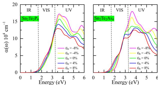
Fig. 5 Effect of strains ranging from  $-8\%$  to  $8\%$  on the light absorption rate  $\alpha(\omega)$  of (a)  $\text{Sn}_2\text{Te}_2\text{P}_4$  and (b)  $\text{Sn}_2\text{Te}_2\text{As}_4$  monolayers.
