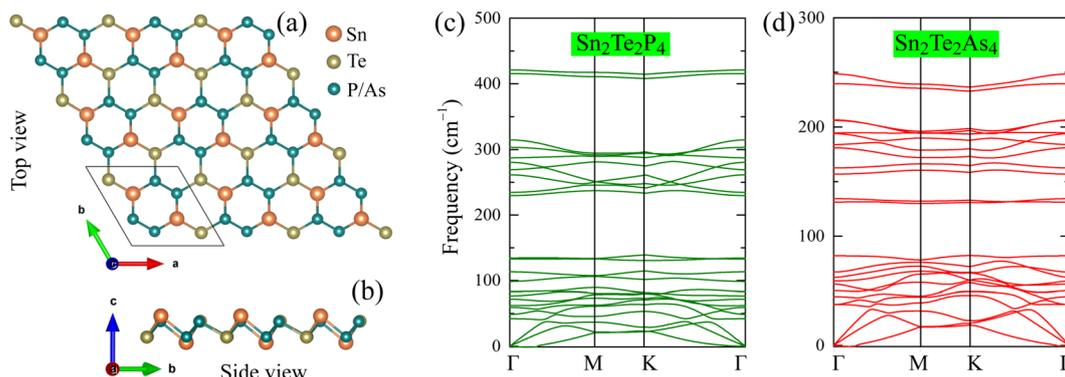
Fig. 1 Atomic structures of  $\text{Sn}_2\text{Te}_2\text{X}_4$  ( $X = \text{P}, \text{As}$ ) monolayers presented in the (a) top view and (b) side view; phonon dispersions of (c)  $\text{Sn}_2\text{Te}_2\text{P}_4$  and (d)  $\text{Sn}_2\text{Te}_2\text{As}_4$ .
