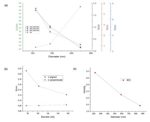
Fig. 10 The reported result of the effect of various diameters of nanofibre on characteristic parameters of PEMFCs, including (a) proton conductivity and activation energy, <sup>69</sup> (b) proton conductivity, <sup>70</sup> and (c) IEC. <sup>71</sup>
