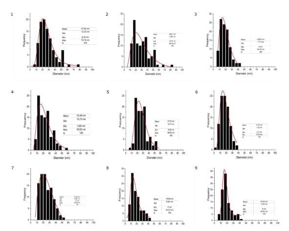
Fig. 5 Measurement of the diameter of nanofibers (mean, standard deviation, minimum, and maximum size are provided)
