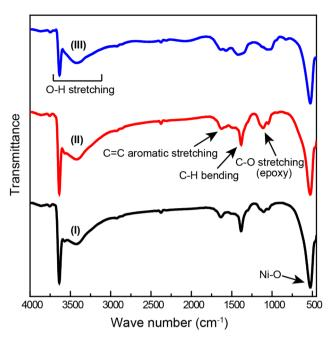
Fig. 5 FTIR spectra of (I) NiO, (II) NiO/CNTs, and (III) Ag/NiO/CNTs showing the functional groups corresponding to CNTs demonstrating the successful formation of the NiO/CNT composite.
