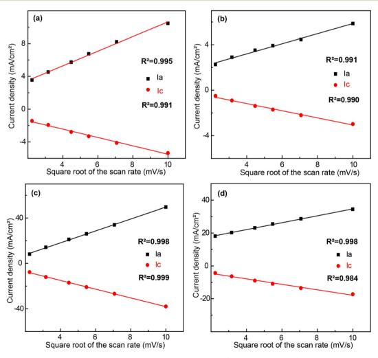
Fig. 7 The evolution of the square root of the scan rate *versus* the peak currents (anodic and cathodic) for the synthesized nanocomposites, namely, NiO (a), NiO/CNTs (b), Ag (25%)/NiO/CNTs (c) and Ag (50%)/NiO/CNTs (d).
