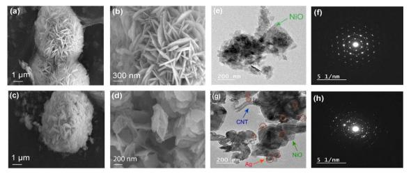
Fig. 3 Electron microscopy imaging for the synthesized catalysts. (a and b) SEM images of NiO nanoflowers with a micro-ball size of  $\sim$ 5  $\mu$ m. (c and d) SEM images of the Ag (25%)/NiO/CNTs catalyst. (e and f) HRTEM imaging and SAED pattern for the as-synthesized NiO. (g and h) TEM images and SAED of Ag (25%)/NiO/CNTs showing the successful synthesis of the doped catalyst with good crystallinity.
