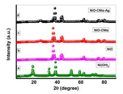
Fig. 1 X-ray diffraction pattern for synthesized nanocomposites. (a) Ni(OH)<sub>2</sub>, (b) NiO, (c) NiO/CNTs, and (d) Ag/NiO/CNTs.
