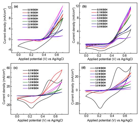
Fig. 8 CVs of the NiO (a), NiO/CNTs (b), Ag (25%)/NiO/CNTs (c) and Ag (50%)/NiO/CNTs (d) at different ethanol concentrations at 50 mV s<sup>-1</sup> scan rate. All cyclic voltammetry measurements were carried out in 1 M KOH.
