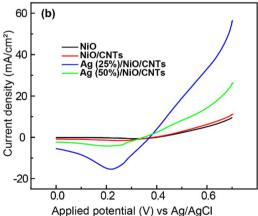
Fig. 9 (a) CVs of the NiO, NiO/CNTs, Ag (25%)/NiO/CNTs and Ag (50%)/NiO/CNTs and (b) its corresponding onset potential with 0.1 mol per L ethanol at a scan rate of 50 mV s $^{-1}$ .
