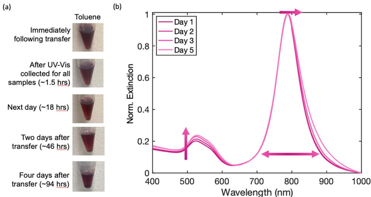
Fig. 4 Visual and spectral data for AuBP sample transferred into toluene as the end solvent. (a) Photographs of AuBP sample in falcon tube. (b) Normalized UV-Vis spectra for corresponding AuBP sample in toluene, exhibiting a relative peak broadening, and red-shift of the long-axis peak, suggesting a slight reduction in stability over time.
