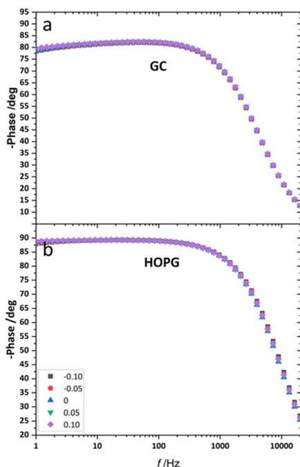
Fig. 8 The example of Bode plot of 20 m LiCl on HOPG (a), and GC (b) from EIS analysis in the frequency range of 20k Hz to 1 Hz at applied potential from  $-0.10$  V to  $0.10$  V (vs. Ag) with  $0.05$  V incremental step.
