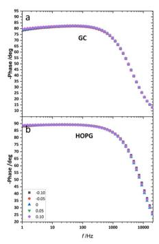
Fig. 8 The example of Bode plot of 20 m LiCl on HOPG (a), and GC (b) from EIS analysis in the frequency range of 20k Hz to 1 Hz at applied potential from -0.10 V to 0.10 V (vs. Aq) with 0.05 V incremental step.
