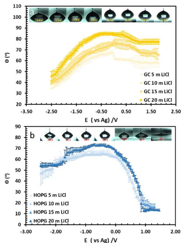
Fig. 4 The change in CA with potential of  $\text{LiCl}$  solution at concentration of 5 m, 10 m, 15 m, and 20 m on GC (a), and HOPG (b). The droplet figures during the electrowetting experiment at 20 m  $\text{LiCl}$  shown on top of the graphs.
