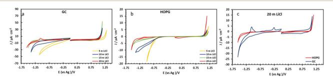
Fig. 3 Cyclic voltammograms of LiCl solution at 5, 10, 15, and 20 m recorded on GC (a) and HOPG (b) surface in PTFE cell set up at scan rate of  $50 \text{ mV s}^{-1}$  respect to Ag pseudo-reference electrode. (c) Shows a comparison of the two electrodes at the highest concentration.
