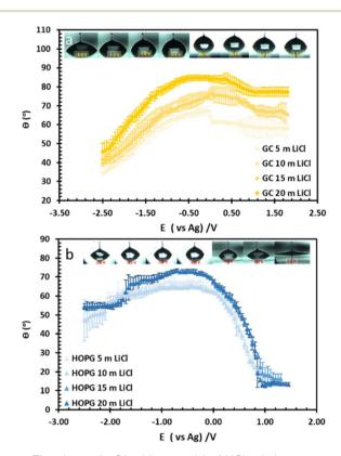
Fig. 4 The change in CA with potential of LiCl solution at concentration of 5 m, 10 m, 15 m, and 20 m on GC (a), and HOPG (b). The droplet figures during the electrowetting experiment at 20 m LiCl shown on top of the graphs
