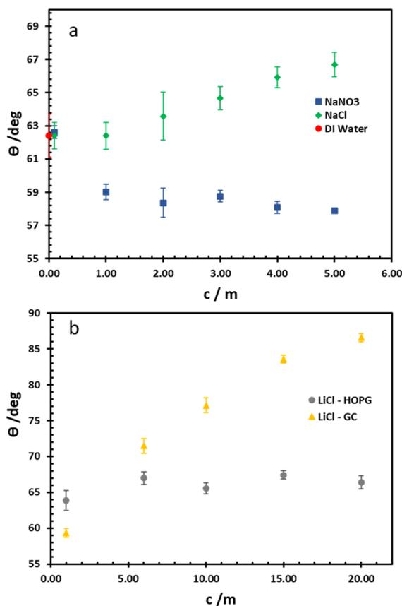
Fig. 2 Equilibrium CA of NaCl and NaNO<sub>3</sub> electrolytes on HOPG (a), and LiCl on both HOPG and GC substrates (b).
