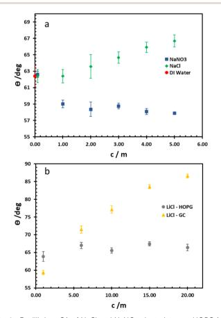
Fig. 2 Equilibrium CA of NaCl and  $NaNO_3$  electrolytes on HOPG (a), and LiCl on both HOPG and GC substrates (b).
