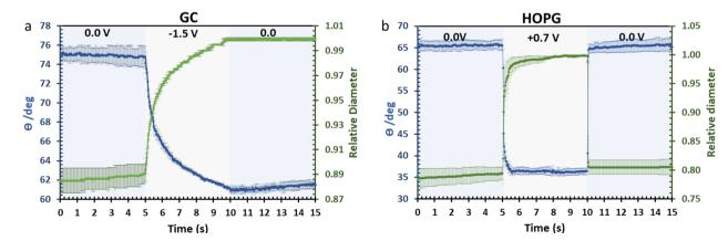
Fig. 9 Dynamic electrowetting on GC (a) and HOPG (b) with negative and positive potential pulse *via* chronoamperometry technique respectively. The changes in CA (blue, left axis) and diameter size (green, right axis) of droplets are then recorded.
