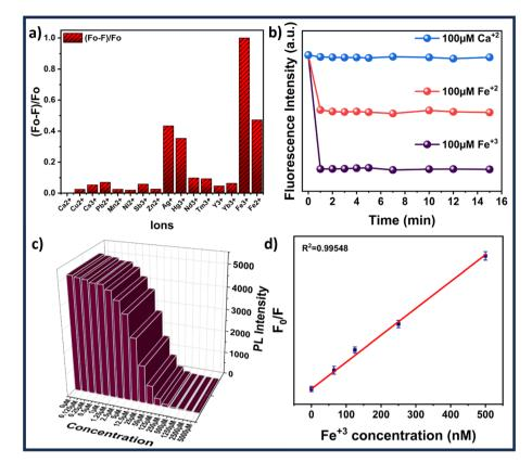
Fig. 5 (a) Bar graph illustrating the fluorescence-based selectivity response of MQDs over a series of different heavy metal ions, (b) the response time optimization of the MQDs after the addition of  $Fe^{3+}$  ions, (c)  $Fe^{3+}$  concentration-dependent fluorescence quenching study of MQDs, (d) linear function describing fluorescence quenching by  $Fe^{3+}$  ions (concentration range 0 nM to 500 nM).
