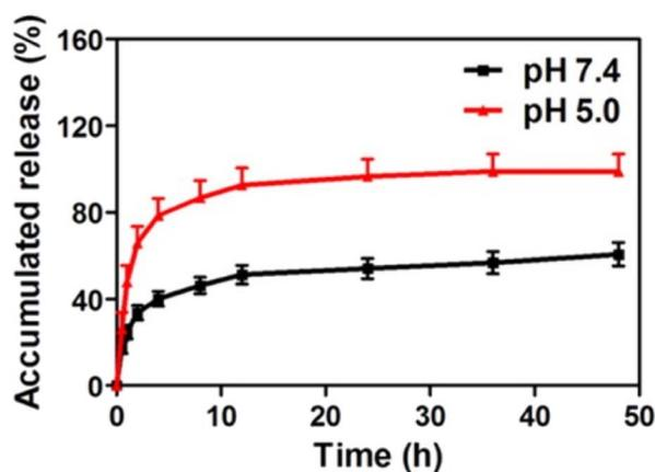
Fig. 7 *In vitro* release profile of DOX-loaded exosomes in pH 5.0 acetate buffer and pH 7.4 phosphate buffer (this figure has been reproduced from ref. 126, with permission from American Chemical Society, Copyright 2016).
