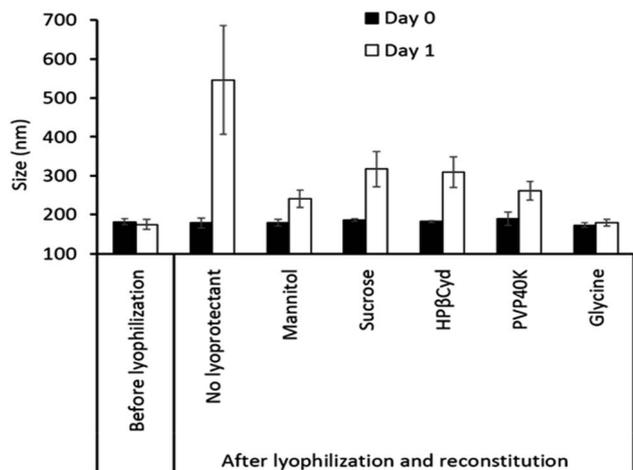
**Fig. 8** Effect of cryoprotectants on the recovery of lyophilized bovine milk-derived exosomes. While original exosomes are stable before lyophilization, the size of lyophilized exosomes without cryoprotectants tripled within 1 day. Using cryoprotectants enhanced the stability of exosomes during lyophilization. Mannitol and glycine 0.5% (w/v) have shown the best effects (cryoprotectant concentration was 0.5% w/v and reconstituted samples were stored at 4 °C).
